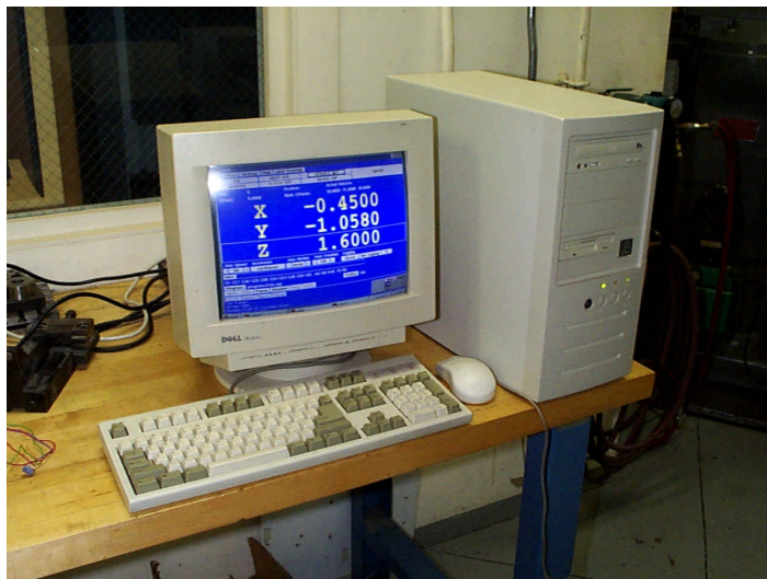
The PC with RTLinux and EMC on it that will control the Bridgeport.
