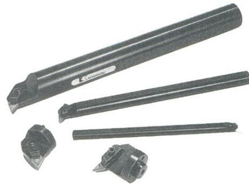
(c) Carbide insert boring bars
