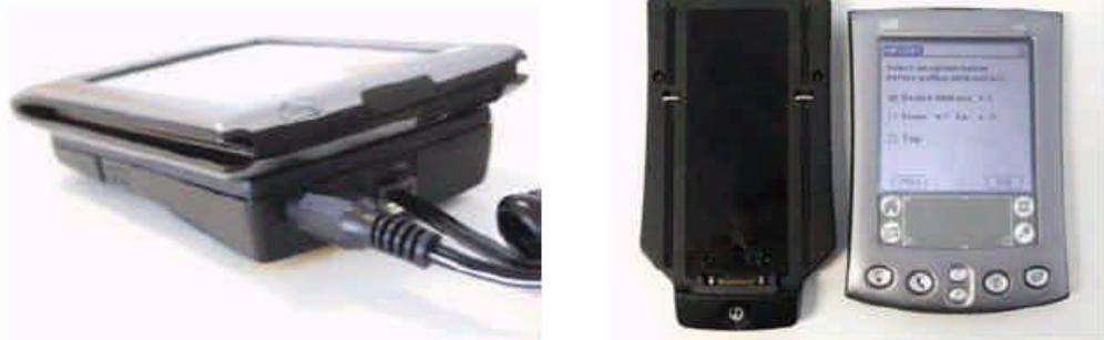
**Figura 5:** Configurador HART: HPC301 e HP311 HART Pocket Interface
