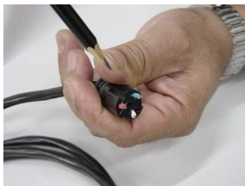
Fig. 1.18 – Wires position in the connector
