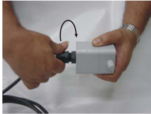
Fig. 1.14 – Disconnecting the cover of the Hall sensor cable
