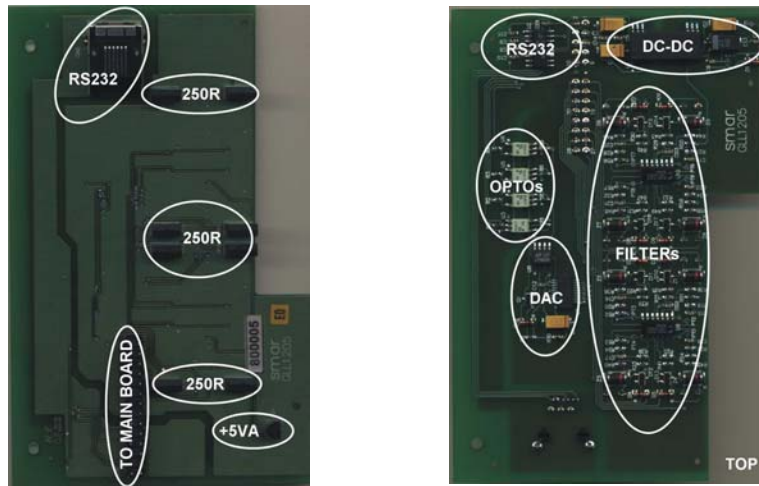
Figure 6.7 – Signal conditioning and low-pass filter circuit
