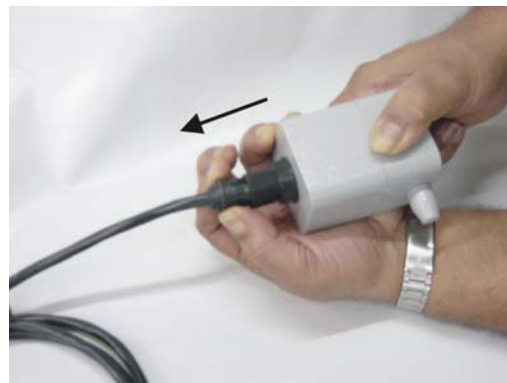
Fig. 1.15 – Disconnecting the Hall sensor cable
