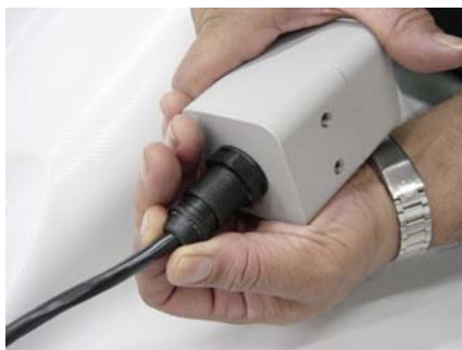
Fig. 1.24– Fasten the cover to the remote Hall.
