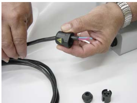
Fig. 1.20 – Assembling the cover
