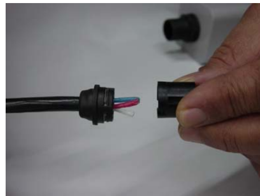
Fig. 1.19 – Release the cables' connector
