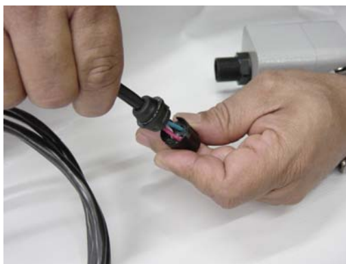
Fig. 1.22 – Inserting the wires in the connector.
