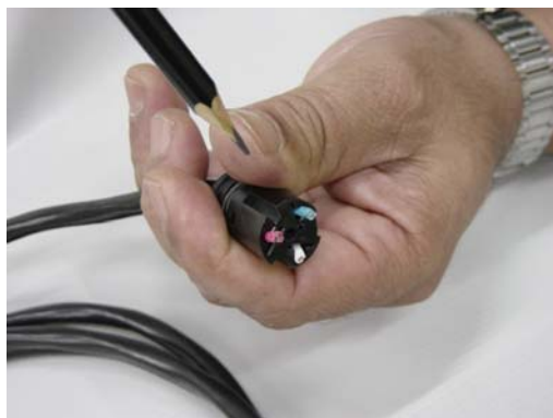
Fig. 1.18 – Wires position in the connector
