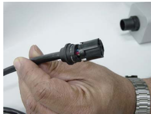
Fig. 1.17 – Connector with the cable's wires maintained in their orifices
