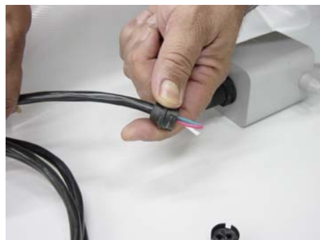
Fig. 1.21 – Assembling the wire bracket
