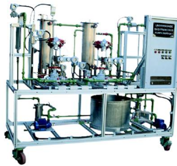
Figure 1. SMAR PD3 Didactic Plant.
