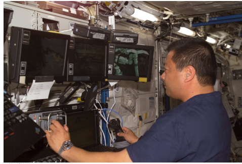
Figure 18 Portion of the workstation that allows controlling Canadarm2 on the ISS. The astronaut manipulates the robotic arm with two joysticks. He has to optimize the limited views offered by the three monitors. (Source: NASA)
