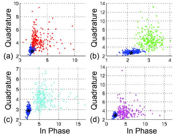
**Fig. 8. Baseline comparisons of the mutual information measure where the baseline distribution (\*) is compared to various states of misalignment and unbalance.**
