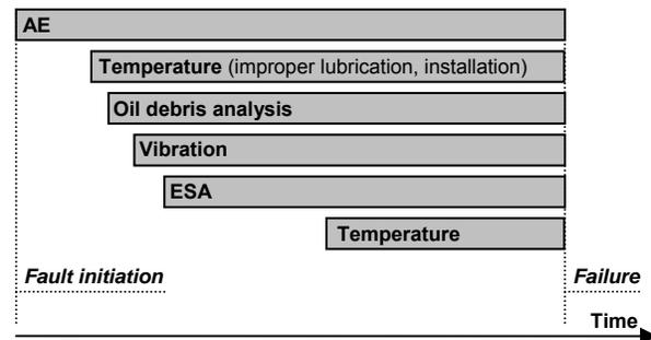
**Fig. 7. Relative comparison of predictive capabilities of the studied measurement methods.**
