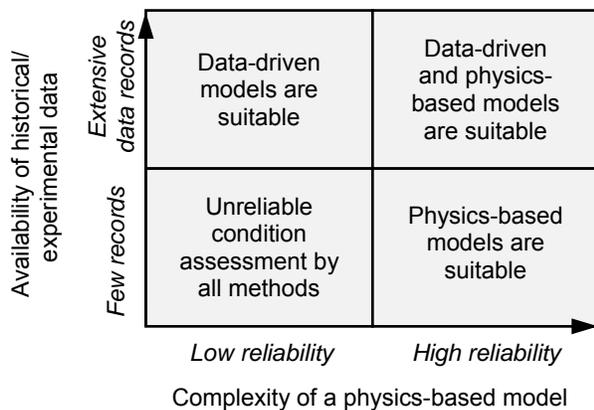
**Fig. 5. Applicability of data-driven and physics-based model techniques for diagnosis and prognosis.**
