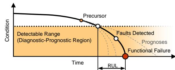
**Fig. 2. Schematic of a component lifetime curve, relating to its condition diagnosis and prognosis.**
