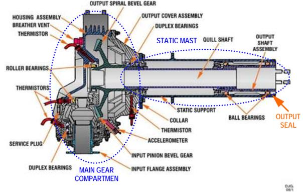
Fig. 9. AH-64 Tail Rotor Gearbox cross section.
