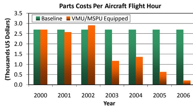
**Fig. 15. Decrease in replaced mechanical components costs for Apache fleet at the SCARNG, due to CBM practice.**
