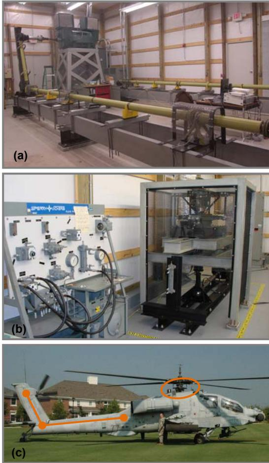
**Fig. 4. USC Tail Rotor Drive Train (a) Test Stand, Main Rotor Swashplate Assembly (b) Test Stand, and Their Correspondence on the Actual AH-64 Helicopter (c).**
