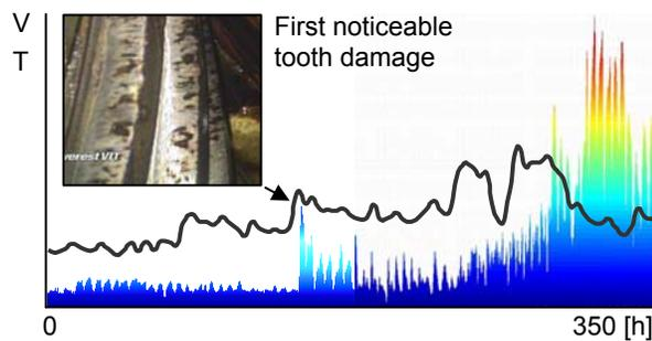
**Fig. 11. Relative maximum vibration level over monitored frequency band, and temperature plots over time.**
