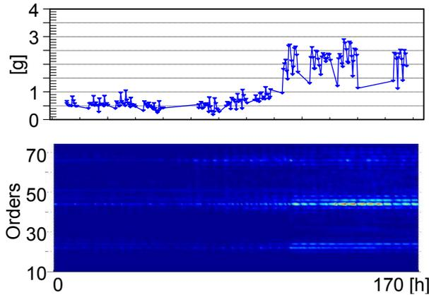
**Fig. 10. TGB Sideband Index CI and vibration order trends over time.**
