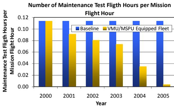
**Fig. 13. Decrease in maintenance test flight hours for Apache fleet at the SCARNG, due to CBM practice.**
