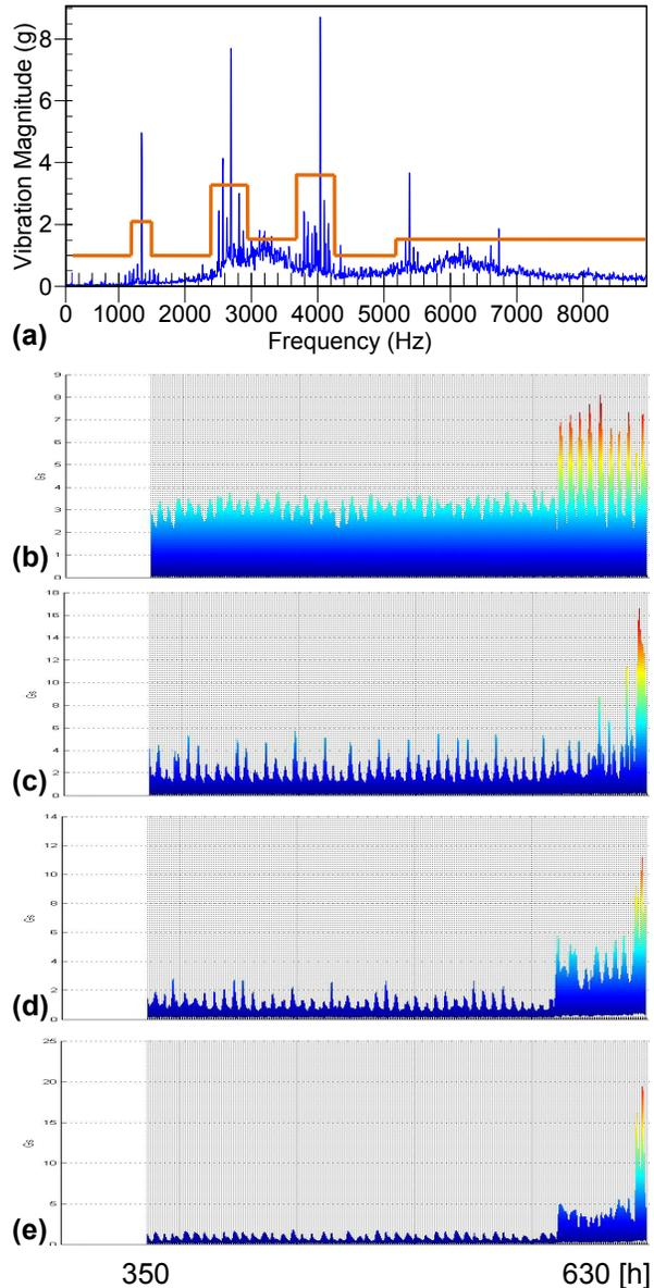
**Fig. 12. Lateral vibrations spectrum over 0-9 kHz frequency band, and its threshold envelope (a); vibration magnitudes at the gear-mesh frequency (1345 Hz) (b), its second (2690 Hz) (c), third (4035 Hz) (e) and fourth (5380 Hz) (d) harmonics, measured at the gearbox duplex input bearing.**
