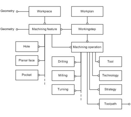
The **Workplan** defines a sequence of **Workingsteps** which associates a certain machining feature with an **Machining Operation**, which in turn describes which type of tool and machining process (drilling, milling, turning etc) that shall be used and its associated strategy.
