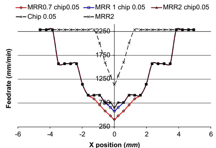
Fig. 10. Feedrate changes rescheduled with various MRR and  $f = 0.05$  mm/rev.
