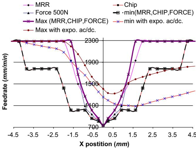
Fig. 12. Feedrate changes with feedrate combination and with exponential ac/deceleration.
