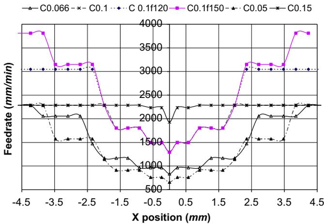
Fig. 3. Feedrate changes with constant chip thickness.
