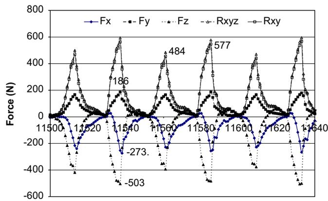
Fig. 5. Cutting forces under  $doc = 3.75$  mm and  $f = 0.05$  mm/rev.
