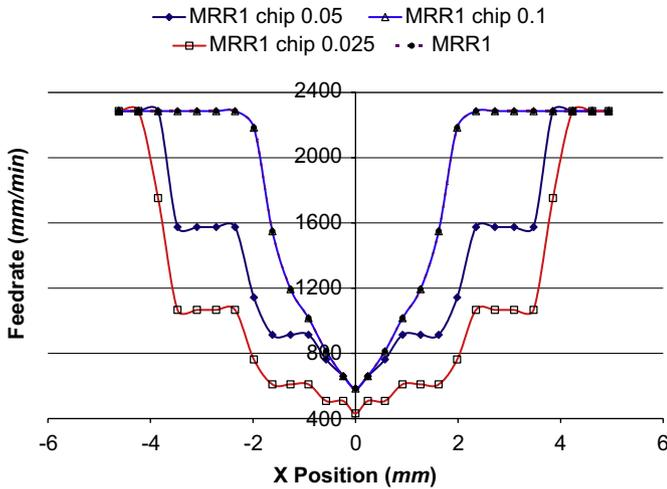
Fig. 11. Feedrate changes rescheduled with various chip thickness and  $MRR = 16387 \text{ mm}^3/\text{min}$ .
