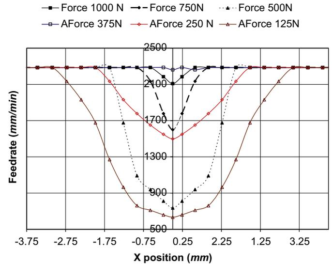
Fig. 7. Feedrate changes with constant resultant forces based on the feed-doc table.
