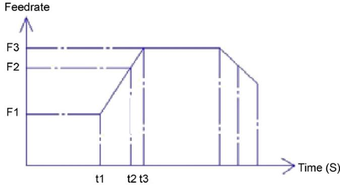
Fig. 1. Time and feedrate considering feedrate ac/deceleration.
