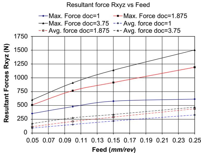
Fig. 6. Relationships between feed and resultant force  $R_{xyz}$ .
