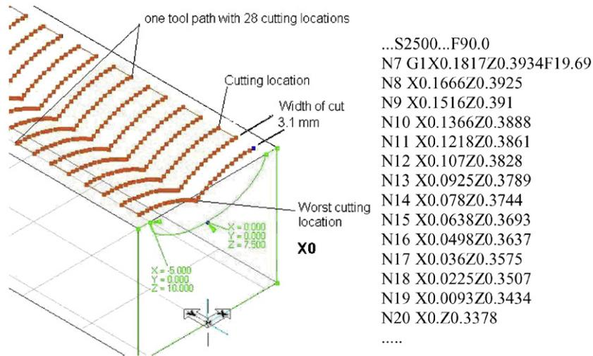
Fig. 2. Tool paths and NC codes for machining a tabulated cylinder.
