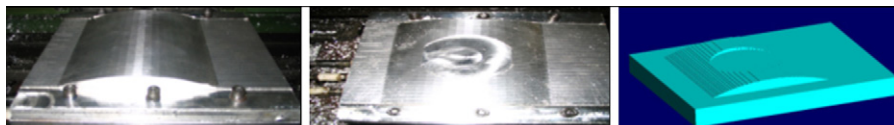
Fig. 10 – View of the circular profile milling. (a) Workpiece before machining, (b) workpiece after machining, (c) output from Oct-OAC.
