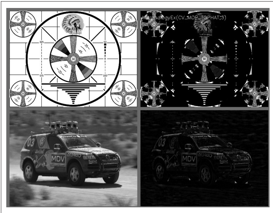
Figure 5-16. Results of morphological Top Hat operation: bright local peaks are isolated
