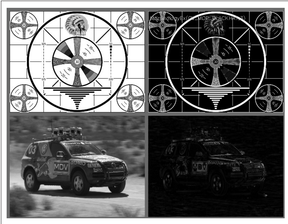
Figure 5-17. Results of morphological Black Hat operation: dark holes are isolated
