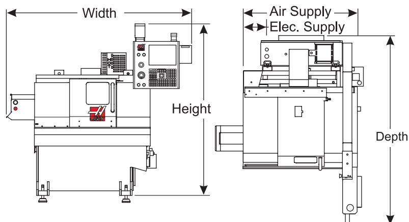
Maximum dimensions of the machine during operation, with the control at its most forward position.
