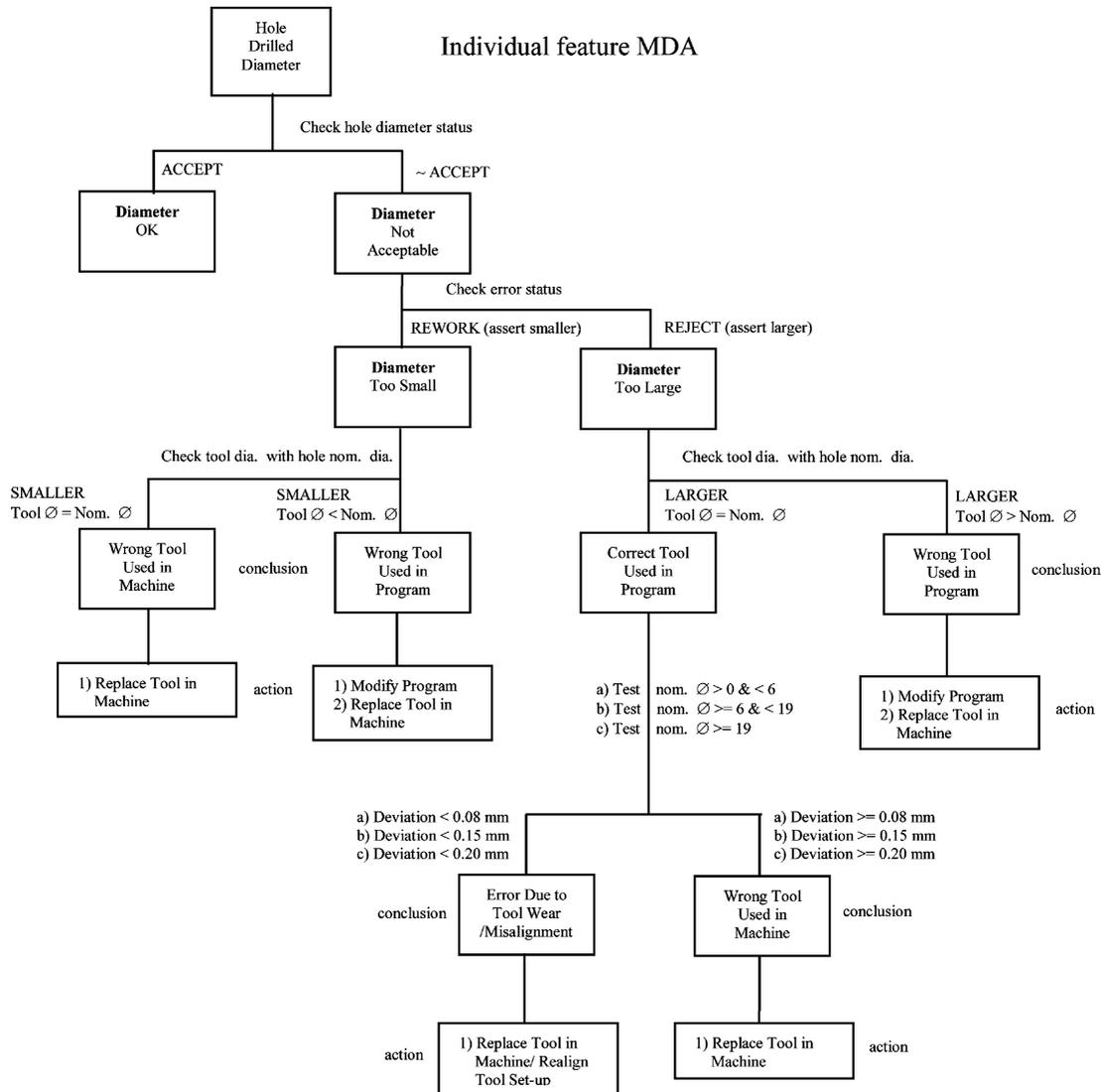
Fig. 2. Logic decision tree for diagnosis of diameter errors of a drilled hole.
