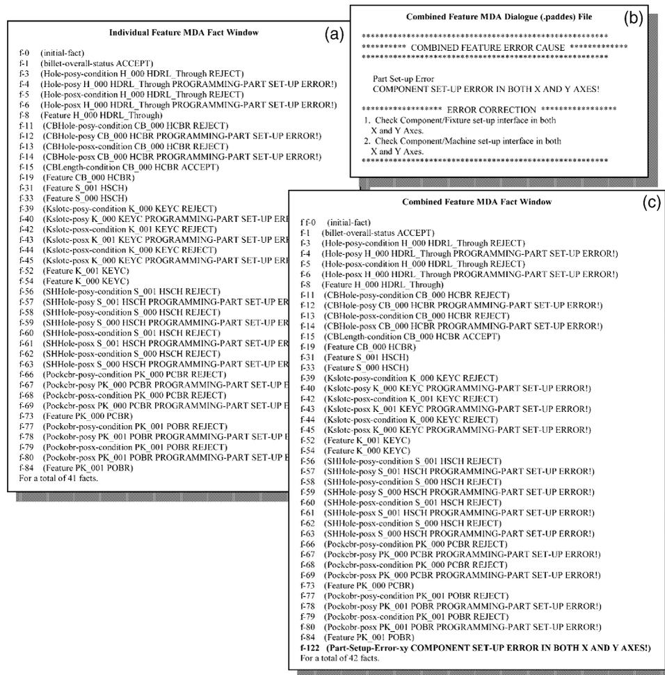
Fig. 9. PADDES consultation output of the combined feature analysis of the component set-up error in both the X and Y axes.
