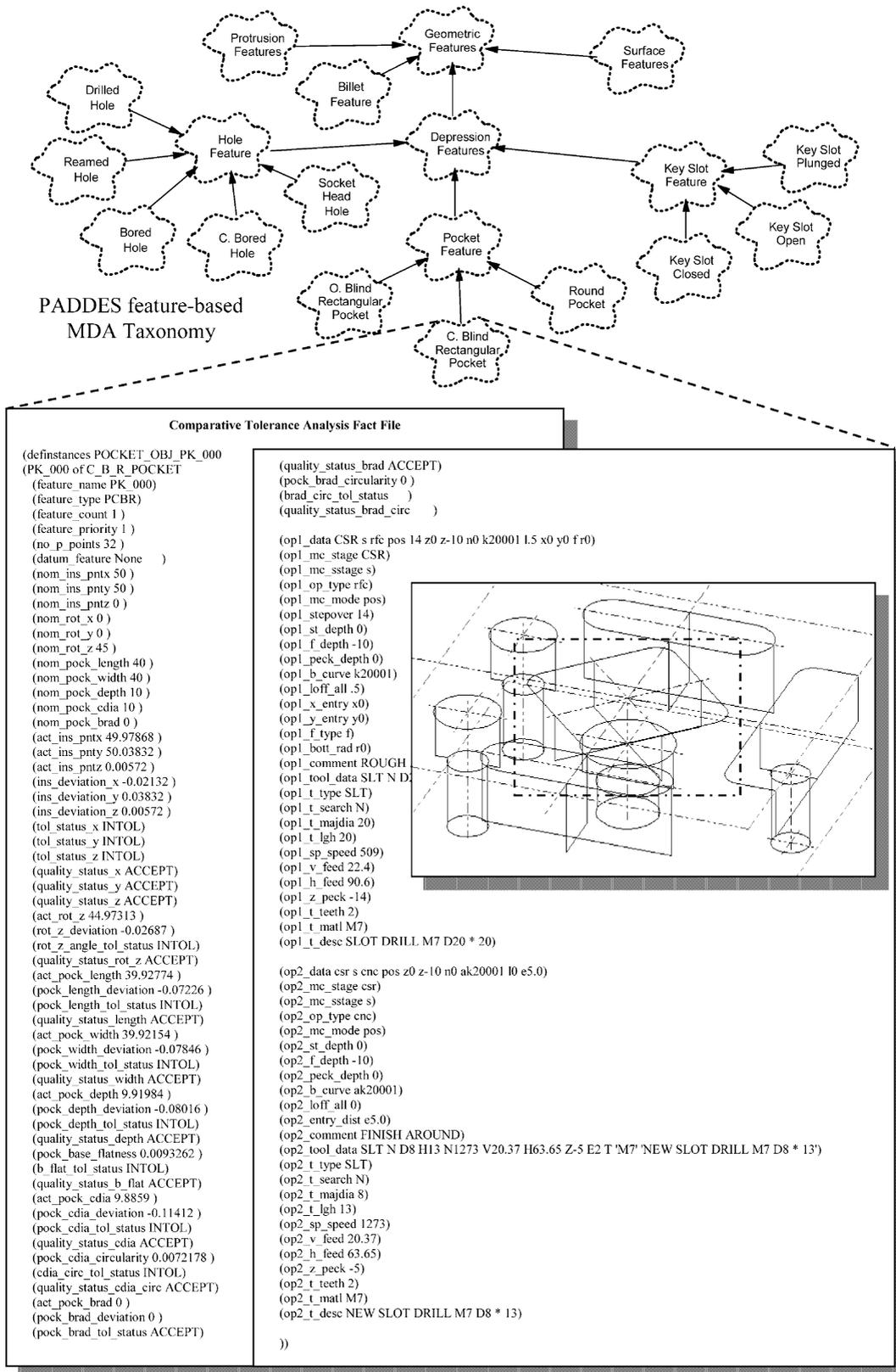
Fig. 4. Comparative tolerance analysis fact file extract for a rectangular feature.
