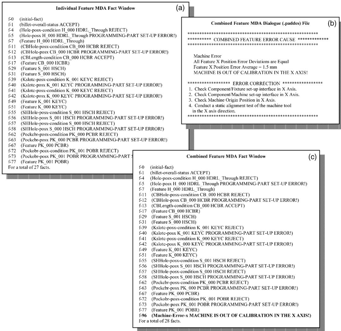
Fig. 8. PADDES consultation output of the combined feature analysis of the machine is out of calibration error scenario of the X axis.
