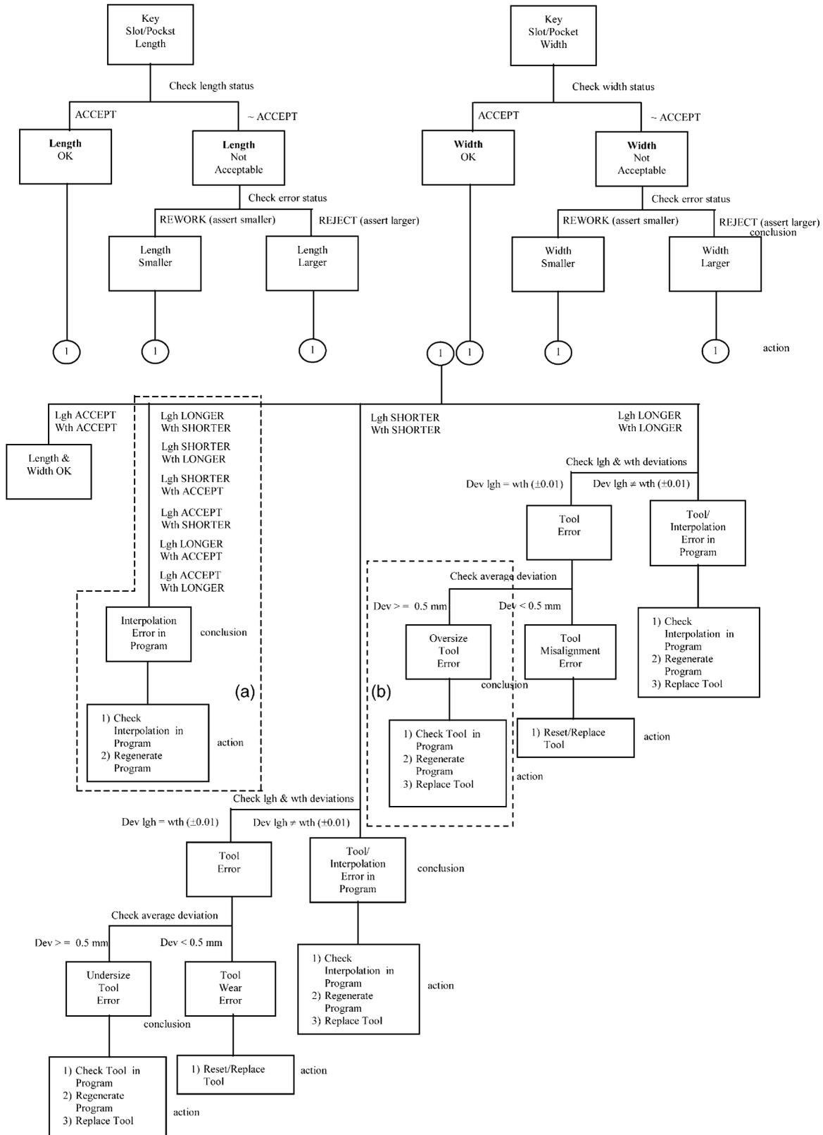
Fig. 5. Logic decision tree for diagnosis of the length and width of a rectangular pocket feature.
