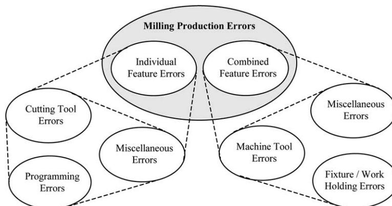
Fig. 1. Feature-based production errors applicable to the milling process.
