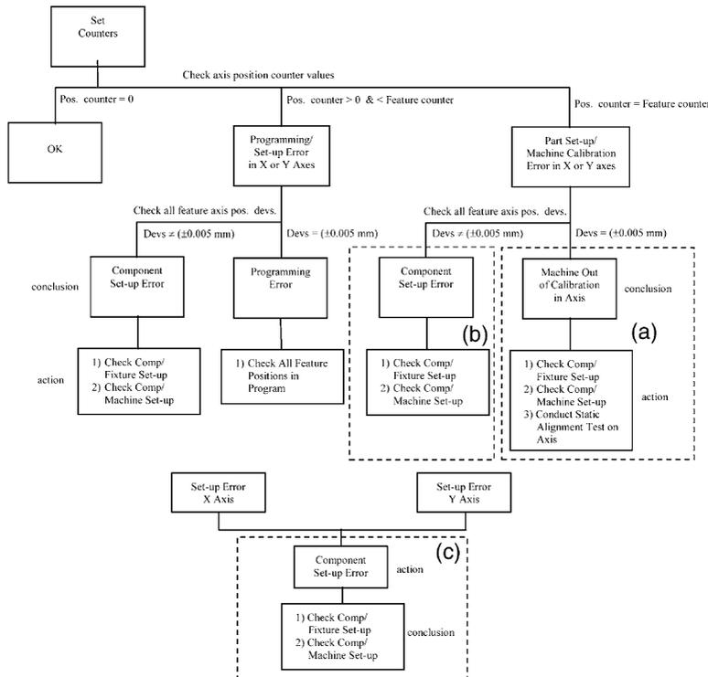
Fig. 7. Logic decision tree for combined MDA diagnosis of the position in the X and the Y axes of the individual feature MDA asserted facts.
