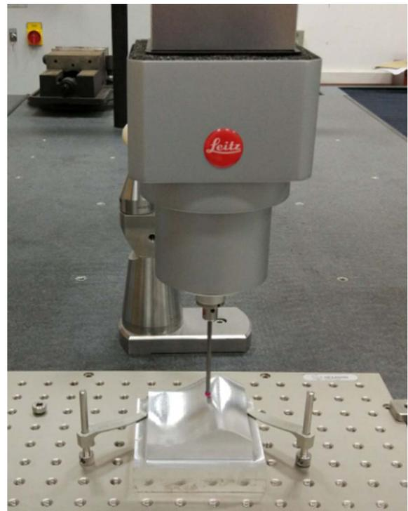
Fig. 9. Offline inspection of the surface part.
