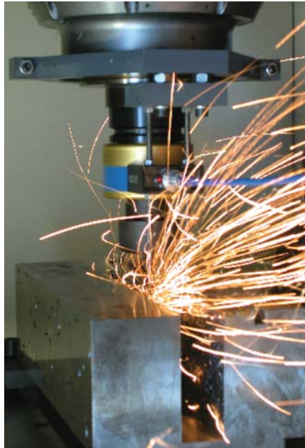
Hard milling (56 HRC) with rotating dynamometer Type 9125A...
