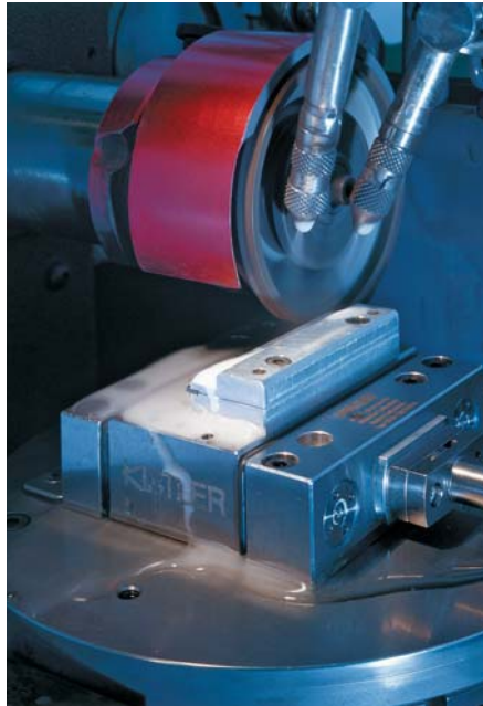
Lateral grinding of silicium workpieces with dynamometer Type 9256C1
