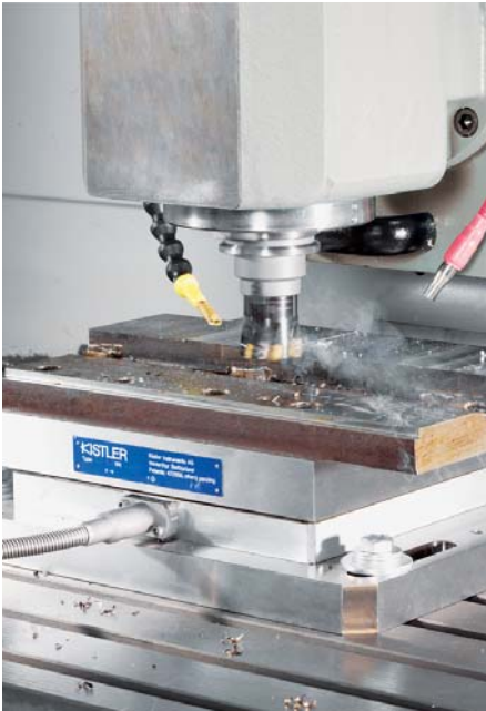
Milling with stationary dynamometer Type 9255B
