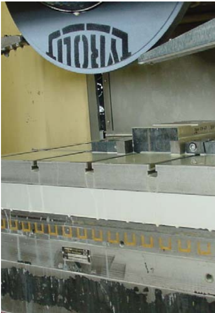
Creepfeed grinding with force plate Type 9253B23
