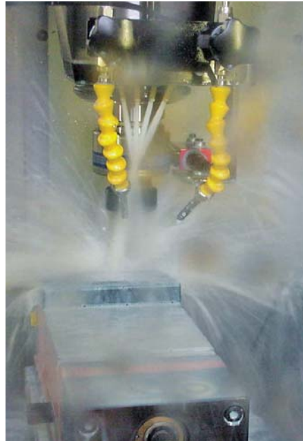
Drilling with the rotating system Type 9125A...
