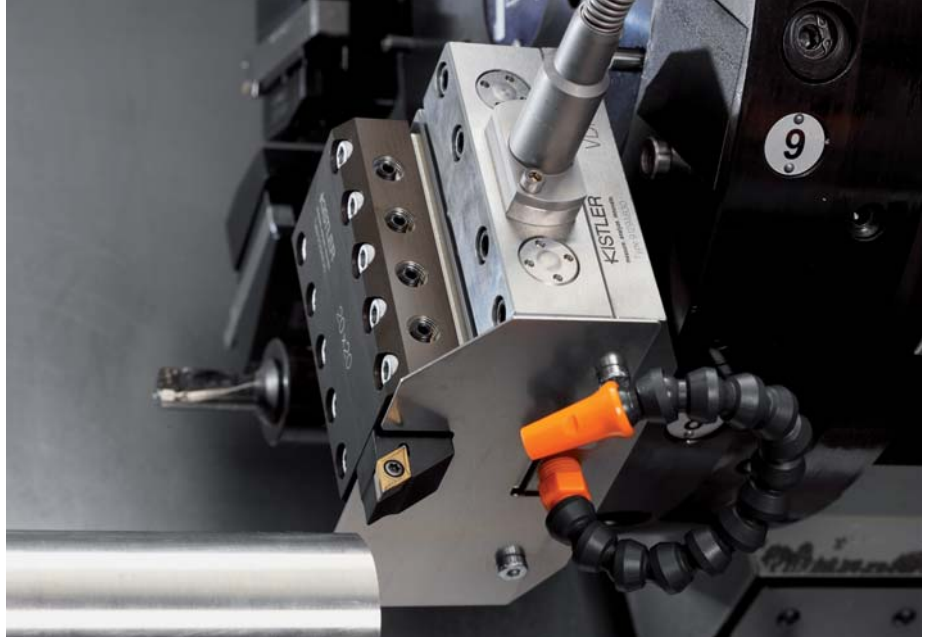
Turning with dynamometer Type 9129A...
