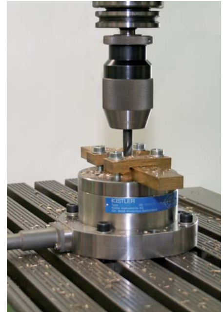
Drilling with stationary dynamometer Type 9272
