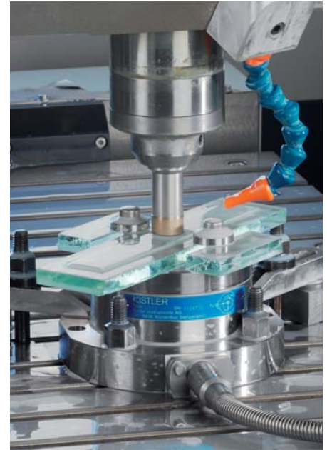
Measurement of forces and torques when drilling the central bore in quartz washers with Type 9272
