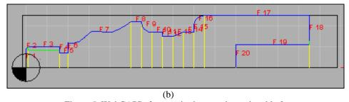
Figure 5. WebCAPP: features in the part shown in table 2.
