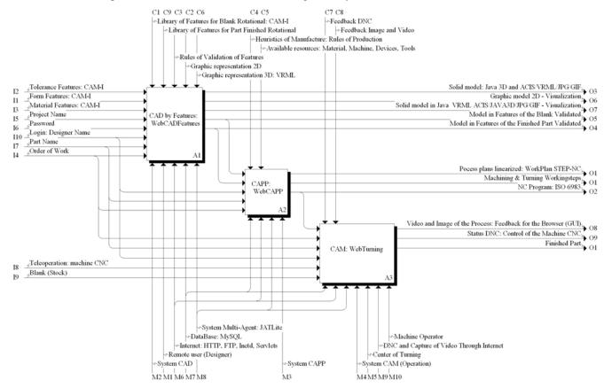
Figure 1. WebMachining: IDEF0 Model (http://webmachining.alvarestech.com/idef0/report\_idef0/index.html).
