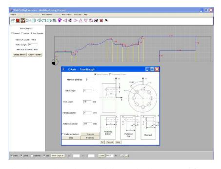
Figure 18. Example2 part is composed of concentric and non-concentric features.
