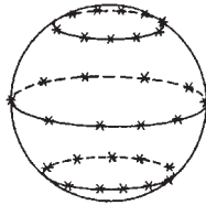
Fig. 18.107 Distribution of N = 30 points on a spherical surface of r = 100 mm and h = 150 mm, so that n_c = 3 and n_p = 10
