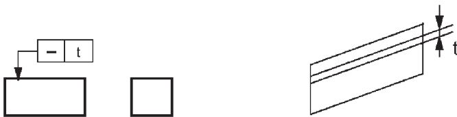
Fig. 3.15 Tolerance zone between two parallel straight lines in a plane
