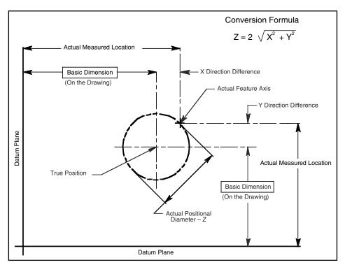
Figure A.1 Conversion diagram from coordinate measurements to cylindrical tolerance. (The Coordinate Conversion Table is on the next page.)
