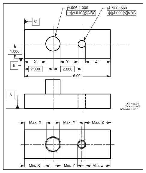
Figure 7-9 The maximum and minimum distances between features.
