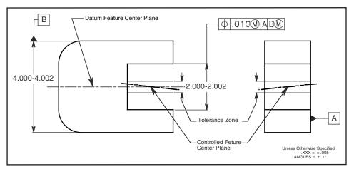
Figure 8-24 A position tolerance used to control the symmetry between size features.
