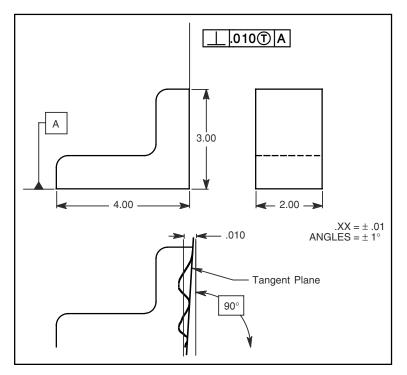
Figure 6-7 Tangent plane specified in the feature control frame.
