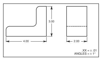
Figure 6-20 Perpendicularity of a plane surface—Problem 2.
