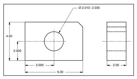
Figure 14-1 A size feature located to plane surfaces on an untoleranced drawing.
