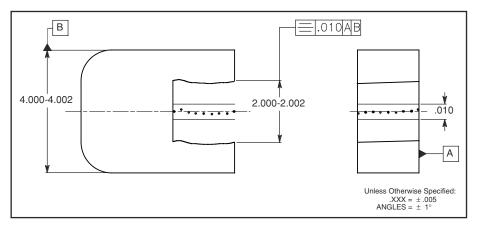
Figure 10-5 A symmetry tolerance locating a symmetrical feature.
