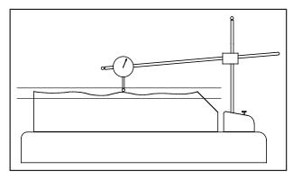
Figure 6-2 Verifying parallelism of a flat surface.
