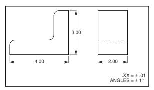
Figure 6-16 Specifying perpendicularity of a surface.
