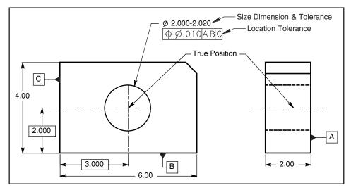
Figure 7-1 Location of a size feature with a position tolerance at RFS.
