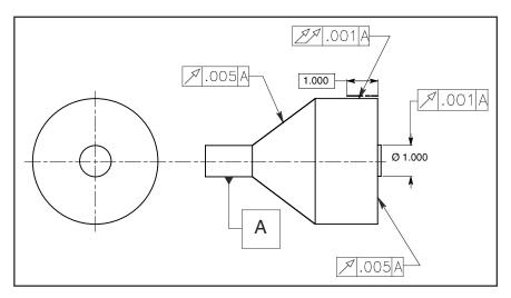
Figure 11-3 Specifying runout and partial runout.
