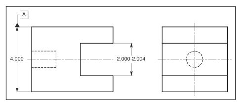
Figure 10-10 Symmetry of the slot: Problem 4.
