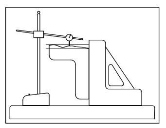
Figure 6-6 Verifying perpendicularity of a flat surface.
