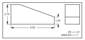
Figure 6-22 Angularity of a plane surface—Problem 4.
