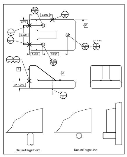
Figure 4-14 A part with datum target areas, target points, and a target line.
