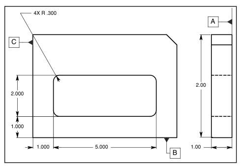
Figure 12-21 A composite profile—Problems 7 through 9.
