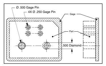
Figure 14-20 A gage locating the four-hole pattern to datum E at MMC and clocking to datum F at MMC.
