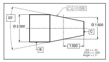
Figure 12-10 Specifying profile of a cone to datum features.
