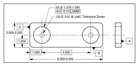
Figure 7-8 Size features toleranced with the LMC modifier.
