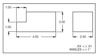
Figure 6-19 Parallelism of a plane surface—Problem 1.
