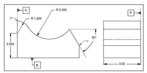
Figure 12-16 Profile of a surface between two points: Problem 2.
