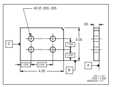
Figure 8-30 Composite tolerancing: Problems 14 and 15.
