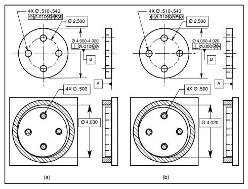
**Figure 7-7** The four-hole pattern, as a group, can shift an amount equal to the difference between the sizes of the outside diameter of the part and the inside diameter of the gage.
