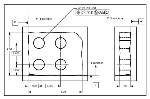
Figure 4-4 A datum reference frame provides measurement origin and direction.
