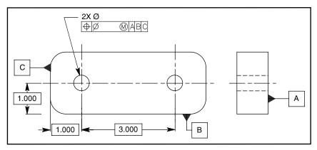
Figure 8-25 Floating fastener drawing: Problems 1 through 4.
