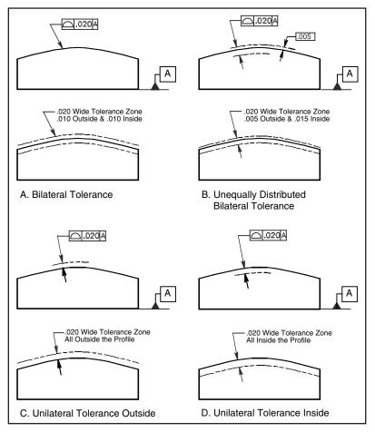
Figure 12-1 Specifying profile of a surface.
