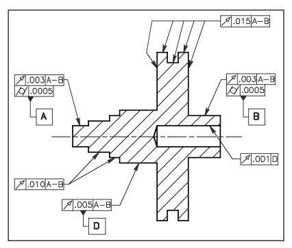
Figure 11-6 Multiple datum features refined with geometric controls.
