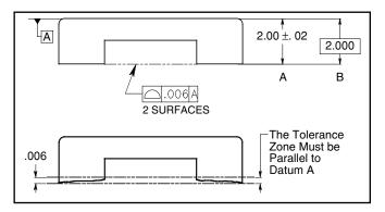
Figure 12-8 Two coplanar surfaces parallel to a datum.
