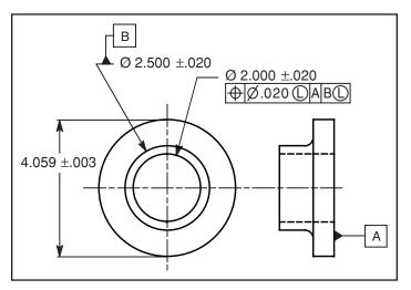
Figure 7-16 A hole specified at LMC: Problem 2.
