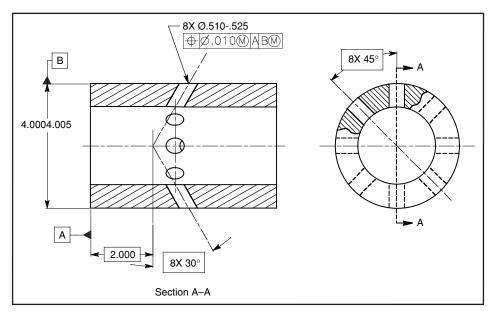
Figure 8-19 Eight holes specified radially about a cylinder and at a  $30^{\circ}$  angle to datum plane A.
