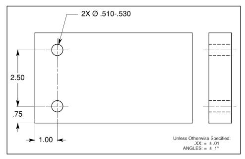
Figure 1-5 No datums are specified on this drawing.
