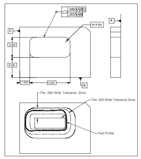
Figure 12-13 A composite profile with two datums repeated in the lower segment.
