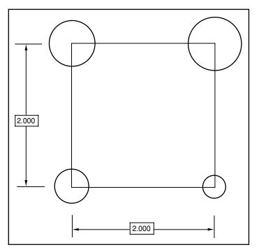
Figure 13-5 The tolerance zone overlay gage.
