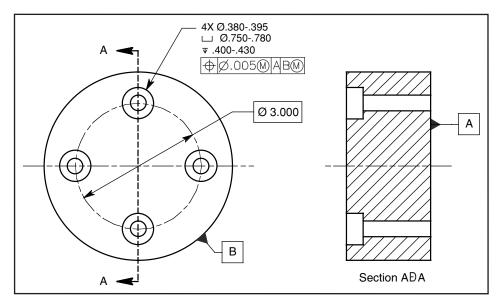
Figure 8-20 Specifications for holes and counterbores with the same tolerances for both.
