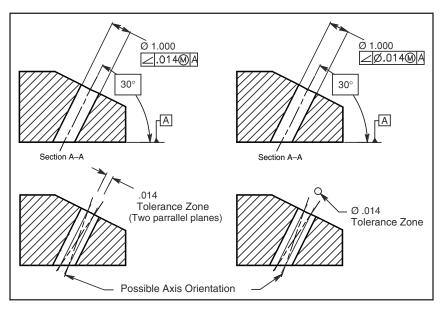
Figure 6-12 Specifying an axis at an angle to a datum plane.
