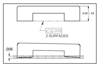
Figure 12-7 Specifying coplanarity with the profile control.
