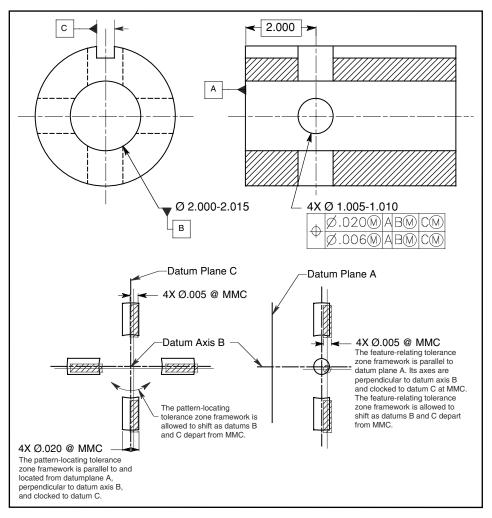
Figure 8-16 A composite positional tolerance with three datums in the upper and lower segments.
