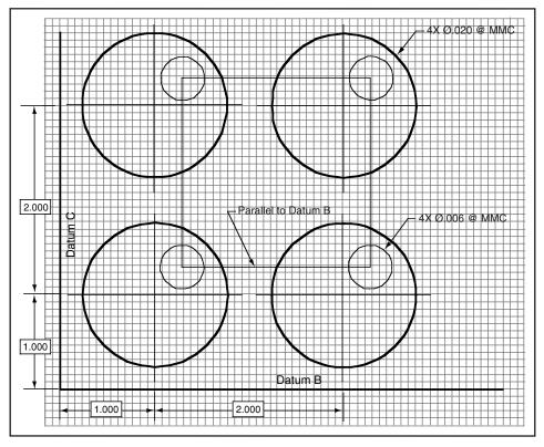
**Figure 8-15** A graphic analysis approach to specifying the datum-to-pattern and feature-to-feature tolerance zone relationships with datums A and B repeated in the lower segment of the feature control frame specified in the drawing in Fig. 8-14.
