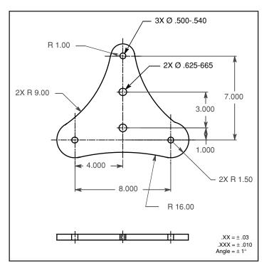
Figure 12-20 Profile controlled to size feature datums: Problem 6.
