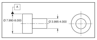
Figure 10-7 Coaxiality of a cylinder: Problem 1.
