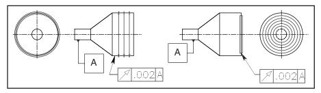
Figure 11-1 Circular runout applied around a datum axis and perpendicular to a datum axis.
