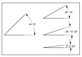
Figure 2-1 Angular measurement expressed with decimals and degrees, minutes, and seconds.
