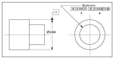
Figure 3-21 Feature control frames specified with RFS and MMC.
