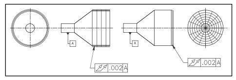
Figure 11-2 Total runout applied around a datum axis and perpendicular to a datum axis.
