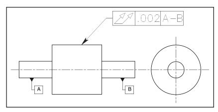
Figure 4-11 Multiple datum features A and B are of equal value.
