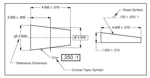
Figure 3-15 Conical taper, slope, and reference dimension symbols.
