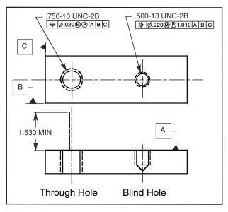
Figure  $8\mathchar`-7$  Specifying projected tolerance zones for through and blind holes.
