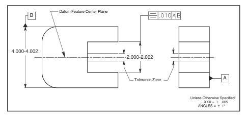
Figure 10-4 The symmetry tolerance zone consists of two parallel planes.
