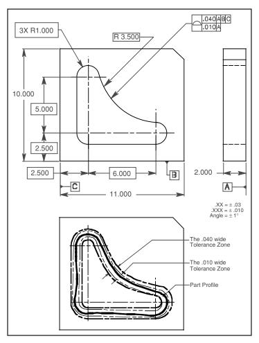
Figure 12-11 A feature controlled with composite profile tolerancing.
