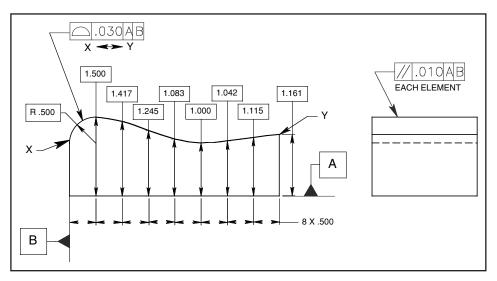
Figure 12-5 Profile refined with a parallelism control of each line element in the surface.
