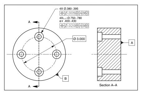
Figure 8-21 Specifications for holes and counterbores with a larger tolerance for the counterbores.
