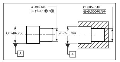
Figure 9-6 Plug and socket.
