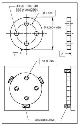
Figure 7-4 Inspecting the hole pattern controlled to a datum feature of size at RFS.
