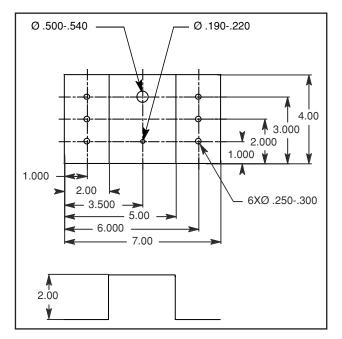
Figure 12-22 The profile of a sheet metal part: Problem 10.
