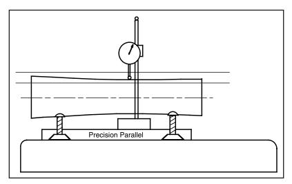
Figure 5-5 Inspection of straightness of a surface.
