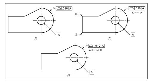
Figure 12-2 The "all around" and "between" symbols and the "ALL OVER" note.
