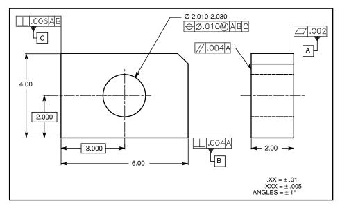
Figure 14-5 Datums controlled for form and orientation.
