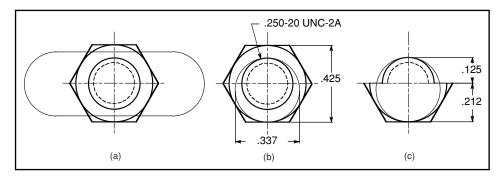
Figure 8-3 Clearance hole size at LMC.
