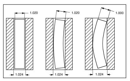
Figure 5-7 Inspection of straightness of a size feature at MMC.
