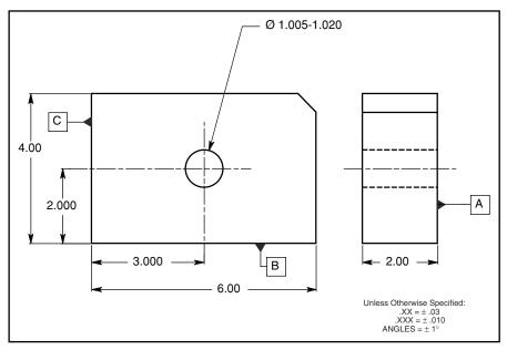
Figure 14-21 A hole located and oriented to datums A, B, and C for questions 1 through 5.
