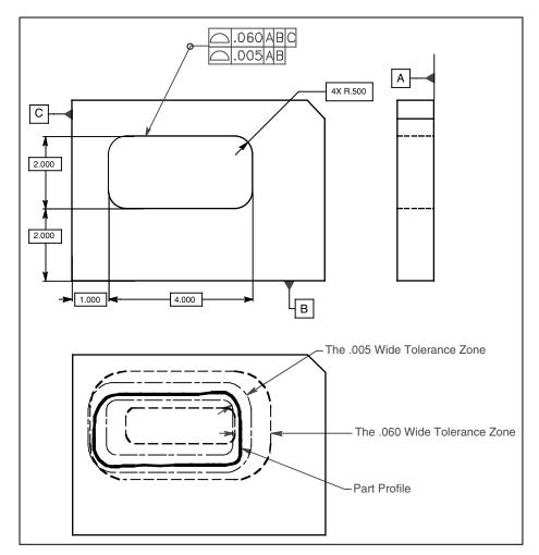
Figure 12-14 A two single-segment profile feature control frame.
