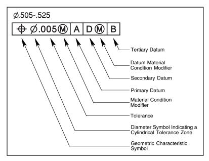
Figure 3-3 The feature control frame explained.
