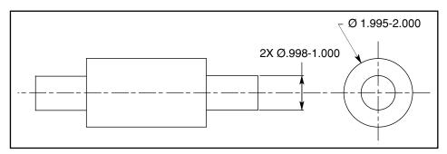
Figure 11-10 Datums toleranced with a cylindricity tolerance: Problem 3.
