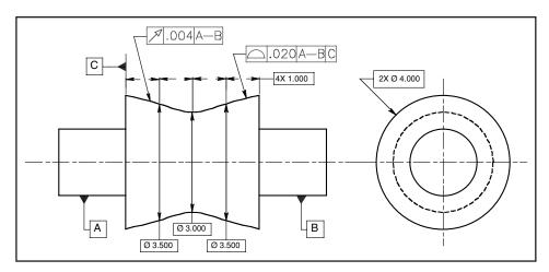
Figure 12-6 A profile refined with a circular runout control.
