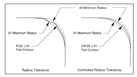
Figure 3-12 Radius and controlled radius tolerances.
