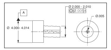
Figure 10-2 A concentricity tolerance locating a coaxial feature.
