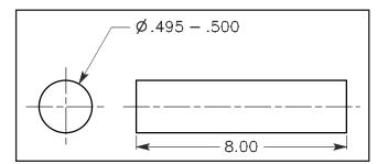
Figure 5-15 Straightness of a median line—Problem 4.
