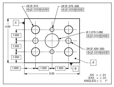
Figure 8-8 Multiple patterns of features located to datum features not subject to size variation (plane surfaces).
