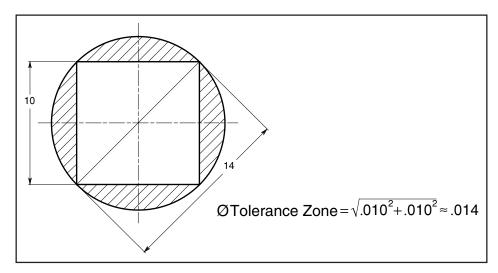
Figure 1-3 A cylindrical tolerance zone provides a uniform distance from the axis to the edge.
