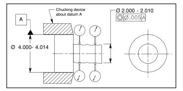
Figure 10-3 Inspecting a part with a concentricity tolerance.
