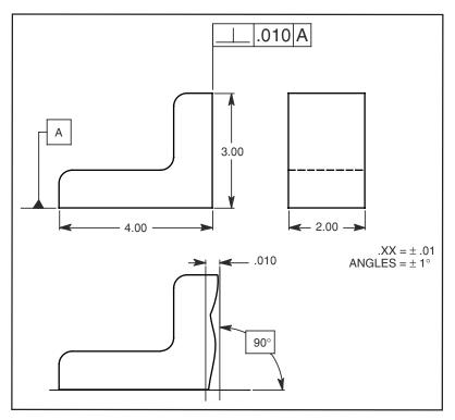
Figure 6-5 Specifying a plane surface perpendicular to a datum plane.
