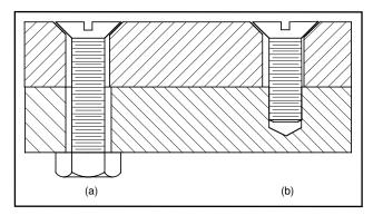
Figure 8-4 A fixed fastener and a double-fixed fastener.
