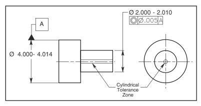
Figure 10-1 Concentricity has a cylindrical tolerance zone and applies at RFS.
