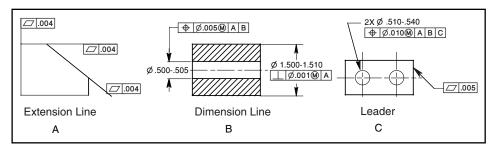
Figure 3-5 Feature control frames attached to features.
