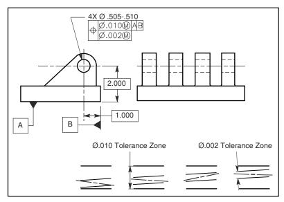
Figure 9-4 Composite control of coaxial features.
