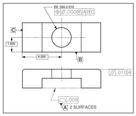
Figure 12-9 Two coplanar surfaces as a datum.
