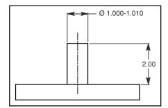
**Figure 6-17** Specifying perpendicularity of a size feature.
