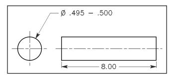
Figure 5-14 Straightness of a surface: Problem 3.
