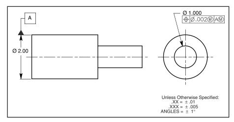
Figure 9-2 Two surfaces of revolution toleranced for coaxiality.
