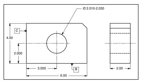
Figure 14-2 A size feature located to specified datums.
