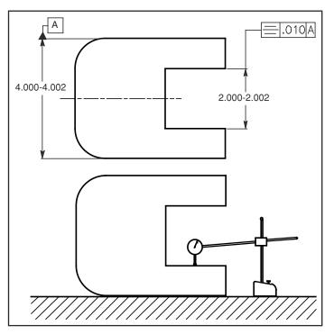
Figure 10-6 Inspecting a part with a symmetry tolerance.
