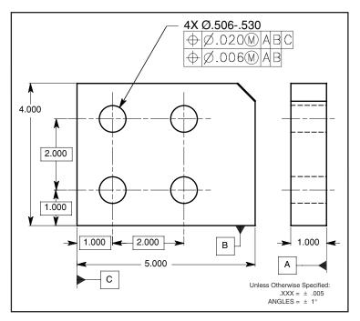
Figure 8-17 A two single-segment feature control frame is used to control a four-hole pattern to datums A and B with a  $\emptyset$ .006 cylindrical tolerance and to datum C with a  $\emptyset$ .020 cylindrical tolerance.
