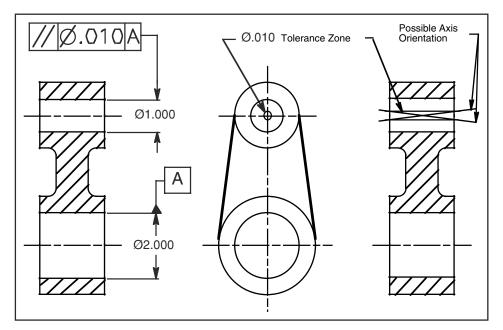
Figure 6-3 Controlling one axis parallel to another axis.
