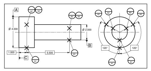
Figure 4-15 Datum targets on a cylindrical part.
