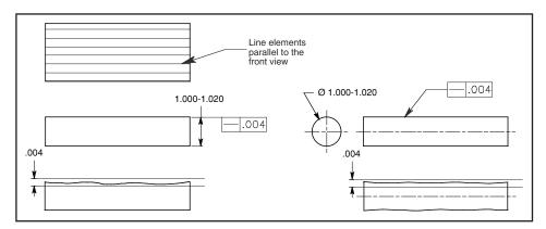
Figure 5-4 Straightness of a surface.
