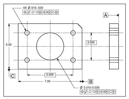
Figure 4-10 Features controlled to datum features of size.
