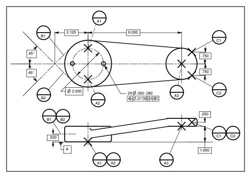
Figure 4-17 Datum targets for step and equalizing datums.
