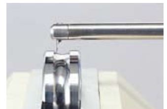
Inner/outer ring contour of a bearing
