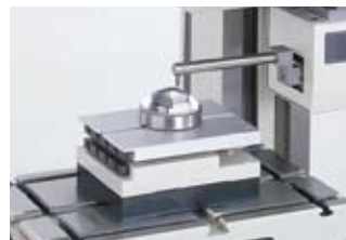
Aspheric lens contour
