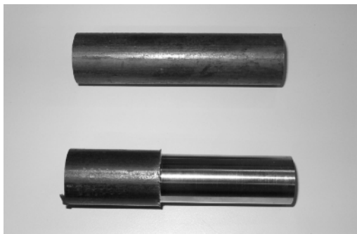
Figure 11.1 Two cylindrical items of the reference case study: a rough piece and a final piece after machining by lathe turning
