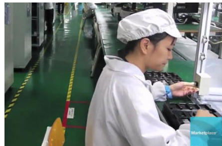
iPad motherboard assembly. Note blue grounding strap on left wrist.
