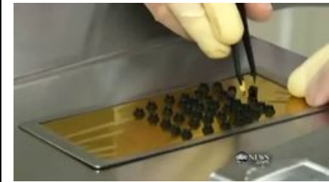
Manually placing components (probably the camera module) on circuit boards. Note gloves, tweezers and bunny suit.
