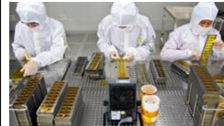
Bunny suits, gloves, ESD work surface and air ionizers for ESD protection.
