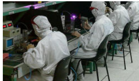
Full bunny suits and ESD grounding straps indicate an effective ESD program and a concern for quality.
