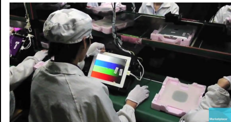
Final testing. No extended burn-in is required, probably because of the extensive ESD control and other quality control.
