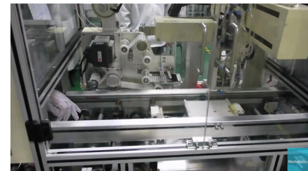
Pick & Place equipment just recently installed.
