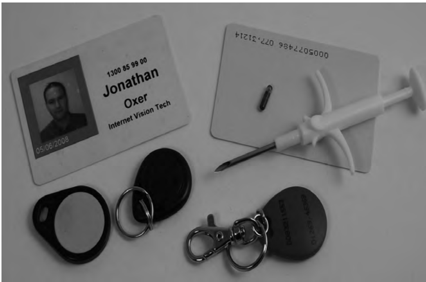
Figure 14-2. RFID tags in a variety of form factors including access cards, key fobs, and a surgically implantable pellet
