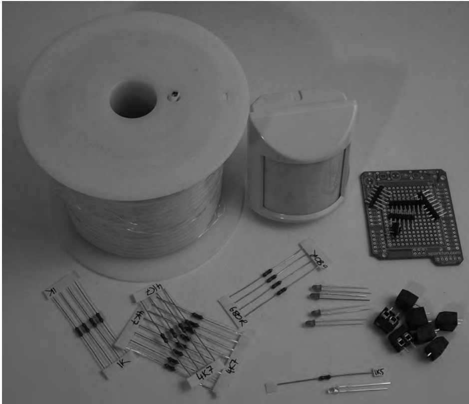
Figure 6-1. Parts required for security sensor inputs
