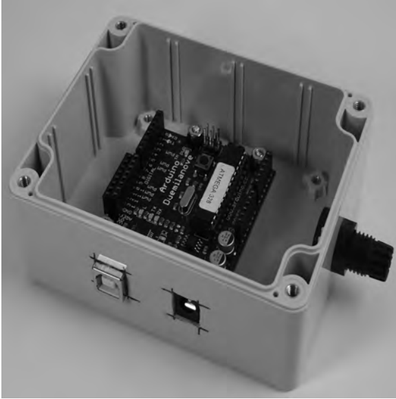
Figure 12-15. Arduino and cable gland mounted in box
