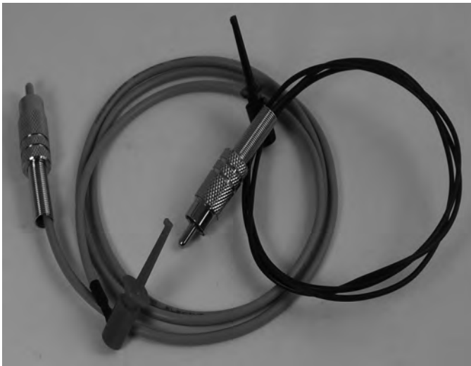
Figure 11-8. Ground probe and test probe
