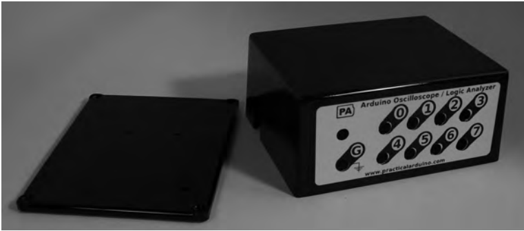
Figure 11-5. Front panel label in place with holes drilled
