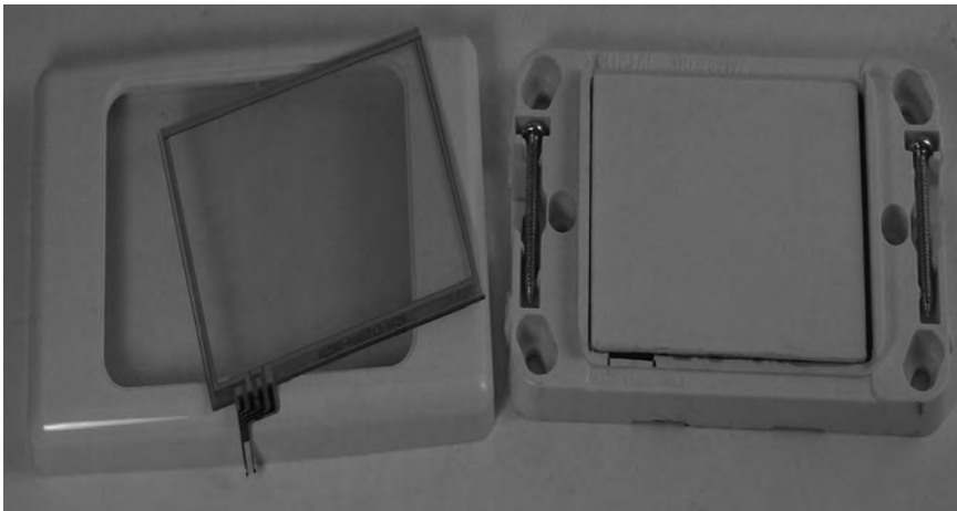
Figure 8-7. Wall plate with removed piece glued back in place behind its original location
