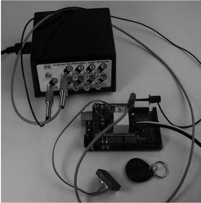
Figure 11-10. Connection to a circuit under test
