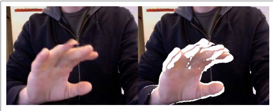
Figure 10-5. Detecting the changed pixels between images
