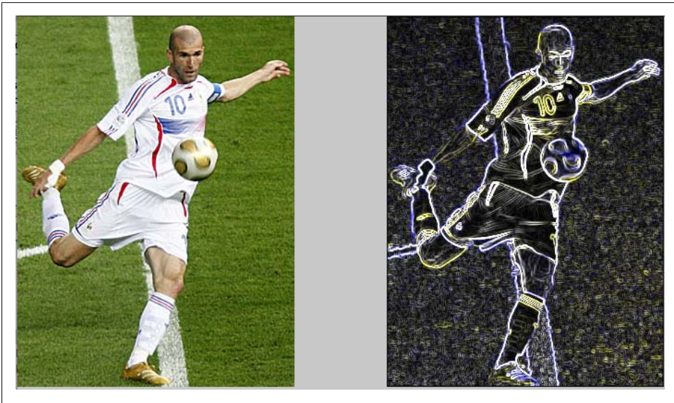
Figure 10-6. Edge detection results on a photo
