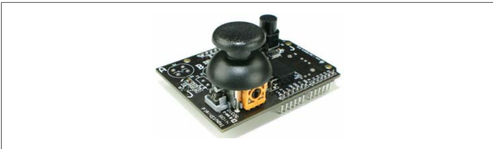
Figure 16-3. The Liquidware InputShield
