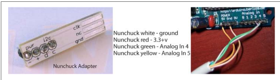
Figure 16-9. Two ways of connecting the Nunchuck to the Arduino: on the left, the Nunchuck Adapter and, on the right, the Nunchuck with the connector removed and wires connected directly to the Arduino
