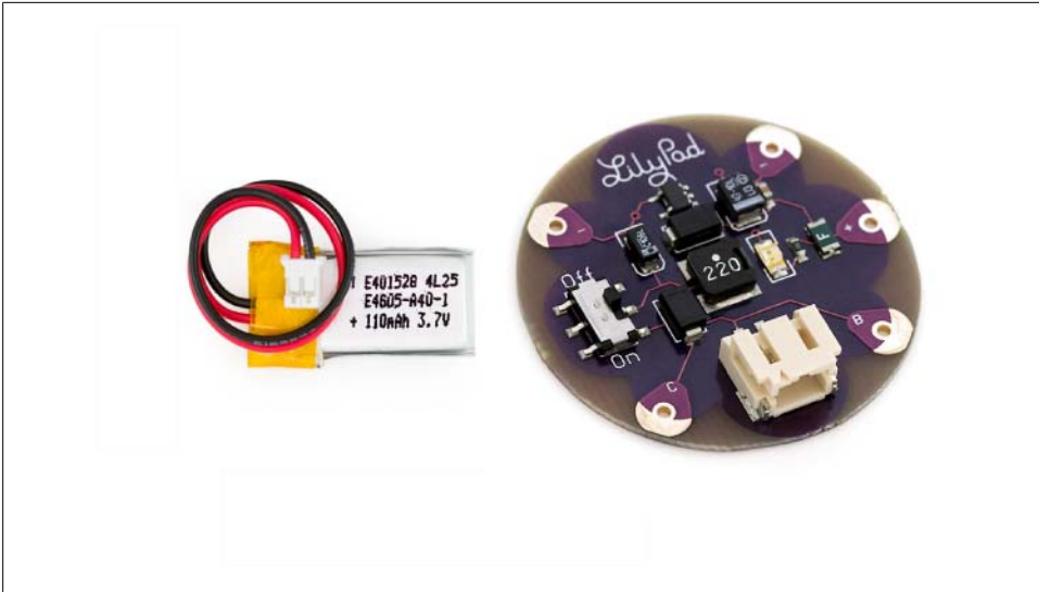
Figure 11-16. Lithium Ion battery and the LiPower board
