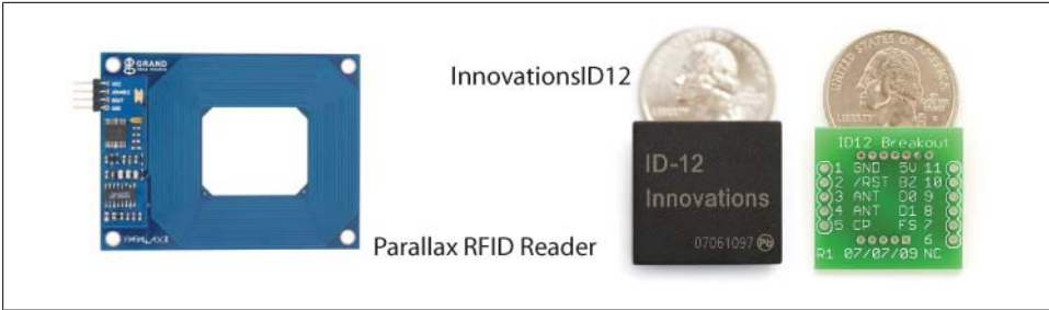
Figure 17-8. RFID readers from Parallax and Innovations
