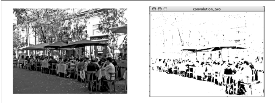
Figure 10-4. Effect of a convolution filter
