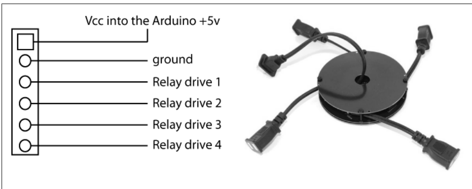
Figure 11-11. The pins on the RelaySquid
