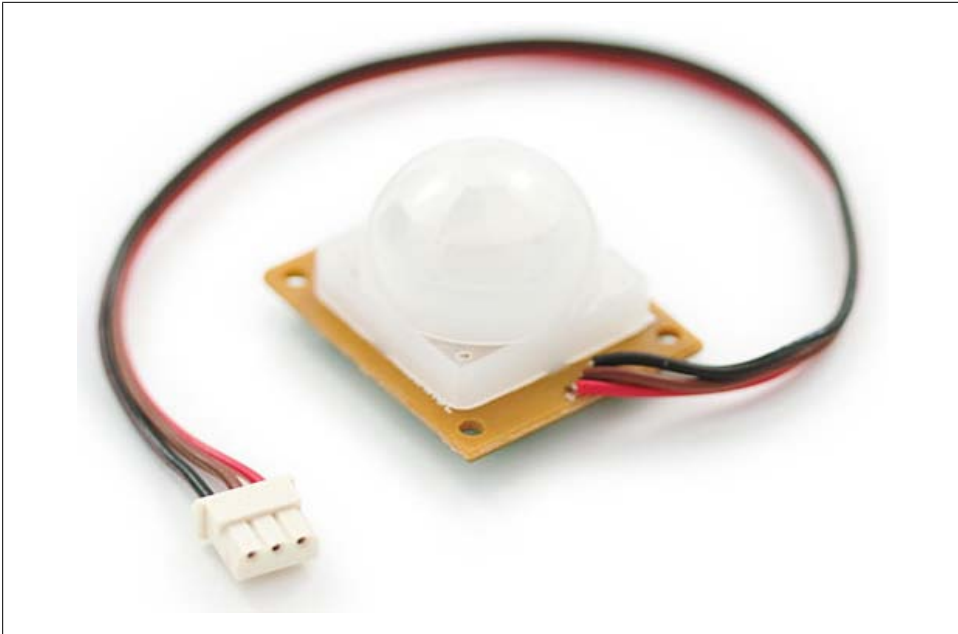
Figure 8-7. PIR motion sensor
