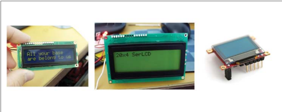
Figure 11-22. A simple 16 × 2 LCD screen, a 20 × 4 LCD, and a Serial Miniature OLED
