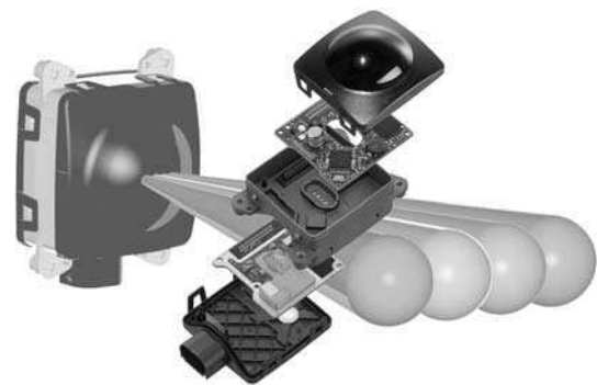
Figure 9.60 Headway sensor and control electronics
