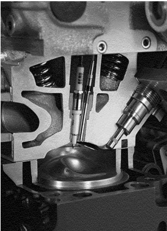
Figure 5.28 Cylinder pressure sensor mounted in the engine
