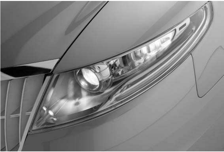
Figure 9.11 Adaptive lighting using LEDs
