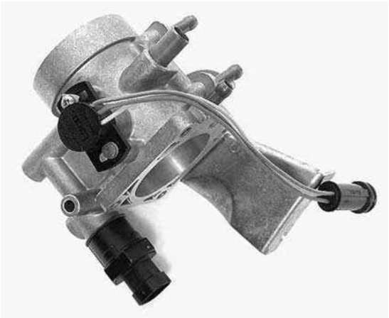
Figure 4.33 Stepper motor and throttle potentiometer on a throttle body
