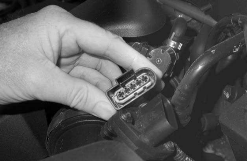
Figure 7.43 Air flow meter under test
