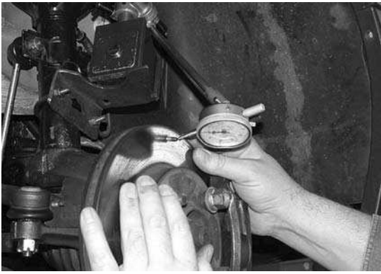
Figure 8.5 Checking a brake disk with a dial gauge
