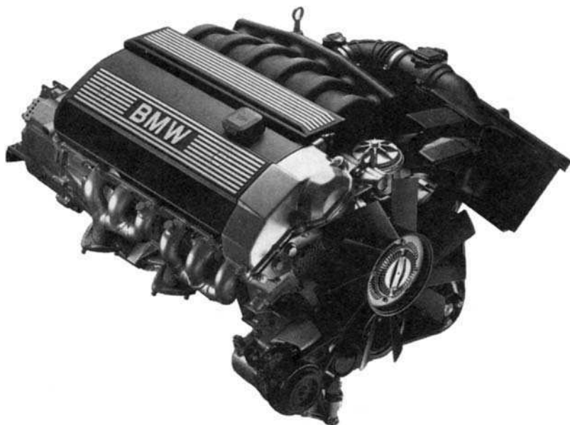
Figure 7.1 The BMW 2.8 litre six cylinder engine uses variable camshaft control
