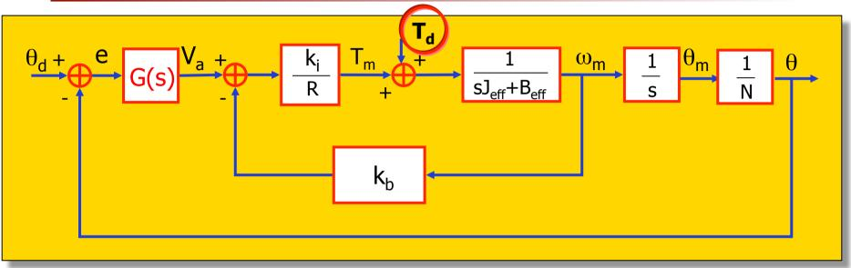
T<sub>d</sub> = disturbance torque due to inertial couplings with other links/axes, centrifugal/Coriolis terms, and gravity (only position-dependent)
