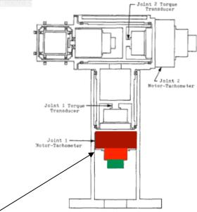
motor, velocity tachometer, optical encoder
