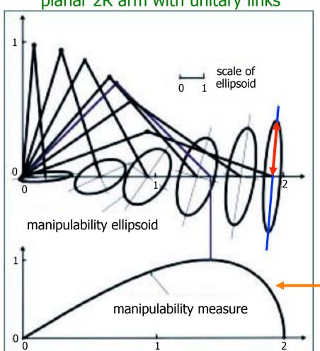
length of principal (semi-)axes: singular values of J (in its SVD)
