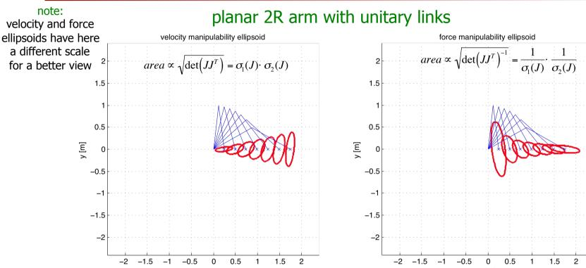
Cartesian **actuation** task (high joint-to-task transformation ratio): preferred velocity (or force) directions are those where the ellipsoid *stretches*
