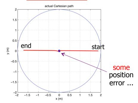
a line from right to left, at  $\alpha$ =179.5° angle with x-axis, executed at constant speed v=0.6 m/s for T=6 s
