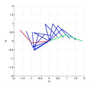
a line from right to left, at  $\alpha$ =170° angle with x-axis, executed at constant speed v=0.6 m/s for T=6 s
