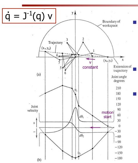
problems arise only when commanding joint motion by inversion of a given Cartesian motion task
