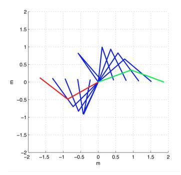
a line from right to left, at  $\alpha$ =178° angle with x-axis, executed at constant speed v=0.6 m/s for T=6 s
