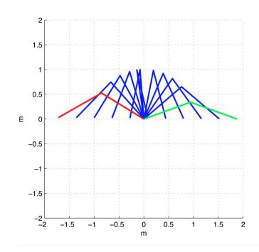
a completely different inverse solution, around/after crossing the region close to the folded singularity
