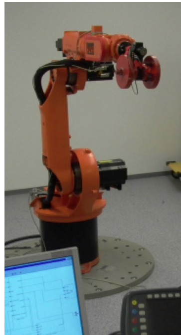
3-axial MEMS accelerometer on the forearm of a KUKA KR15/2 [DLR/Sapienza, 2007]
