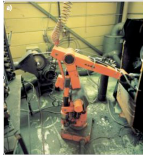
ASEA IRB-6 (1973) first robot all-electric-drives
