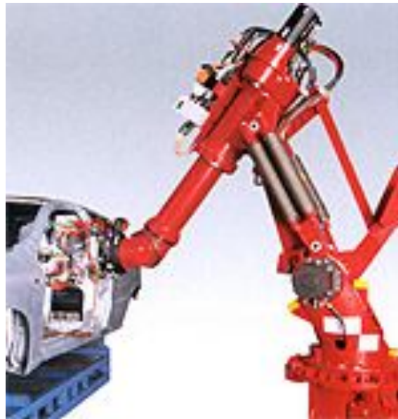
Comau Smart H4 closed kinematic chain
