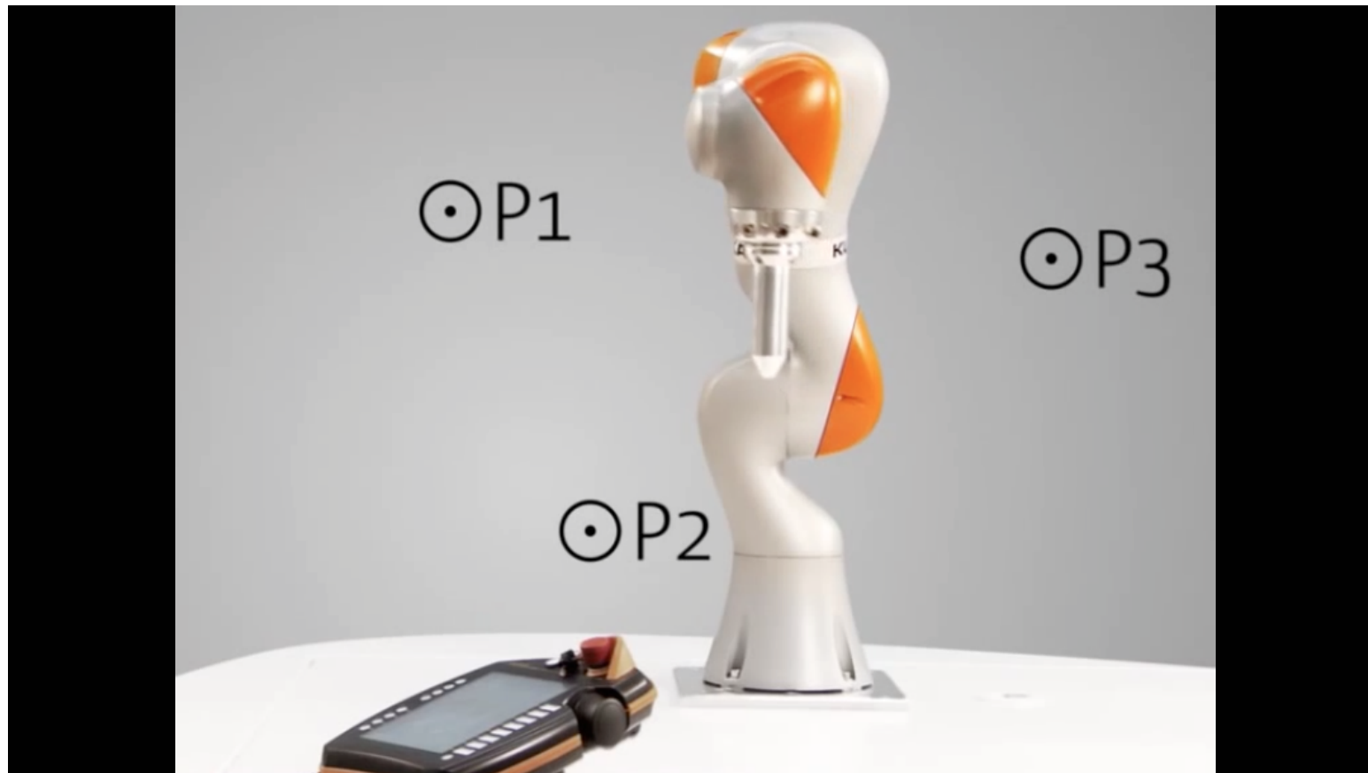
KUKA LBR iiwa robot with 7 revolute joints
