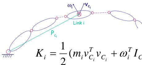
$$K_i = \frac{1}{2} (m_i v_{c_i}^T v_{c_i} + \omega_i^T I_{C_i} \omega_i)$$
