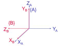
$$R_{ZYX'}(\alpha, \beta, \gamma): \quad \alpha = 0 \\ \beta = 0 \\ \gamma = 90^\circ$$
