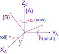
$$R_X(\gamma): v \rightarrow R_X(\gamma).v$$
