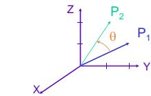
$$P_2 = R_x(\theta) P_1 = \begin{bmatrix} 1 & 0 & 0 \\ 0 & 0.8 & -0.6 \\ 0 & 0.6 & 0.8 \end{bmatrix} \begin{bmatrix} 0 \\ 2 \\ 1 \end{bmatrix} = \begin{bmatrix} 0 \\ 1 \\ 2 \end{bmatrix}$$
