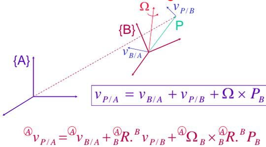
$${}^A v_{P/A} = {}^A v_{B/A} + {}^A R \cdot {}^B v_{P/B} + {}^A \Omega_B \times {}^A R \cdot {}^B P_B$$
