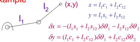
$$\begin{aligned} x &= l_1 c_1 + l_2 c_{12} \\ y &= l_1 s_1 + l_2 s_{12} \\ \delta x &= -(l_1 s_1 + l_2 s_{12}) \delta \theta_1 - l_2 s_{12} \delta \theta_2 \\ \delta y &= (l_1 c_1 + l_2 c_{12}) \delta \theta_1 + l_2 c_{12} \delta \theta_2 \end{aligned}$$
