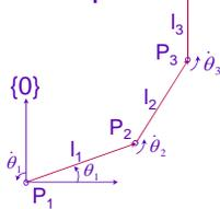
$$v_{i+1} = v_i + \omega_i \times P_{i+1}$$
