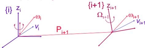
Linear  $v_{i+1} = v_i + \omega_i \times P_{i+1} + \dot{d}_{i+1} \cdot Z_{i+1}$
