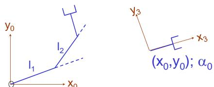
$${}^0_3 T = \begin{pmatrix} c_{123} & -s_{123} & 0 & l_1 c_1 + l_2 c_{12} \\ s_{123} & c_{123} & 0 & l_1 s_1 + l_2 s_{12} \\ 0 & 0 & 1 & 0 \\ 0 & 0 & 0 & 1 \end{pmatrix} = \begin{pmatrix} c\alpha_0 & -s\alpha_0 & 0 & x_0 \\ s\alpha_0 & c\alpha_0 & 0 & y_0 \\ 0 & 0 & 1 & 0 \\ 0 & 0 & 0 & 1 \end{pmatrix}$$
