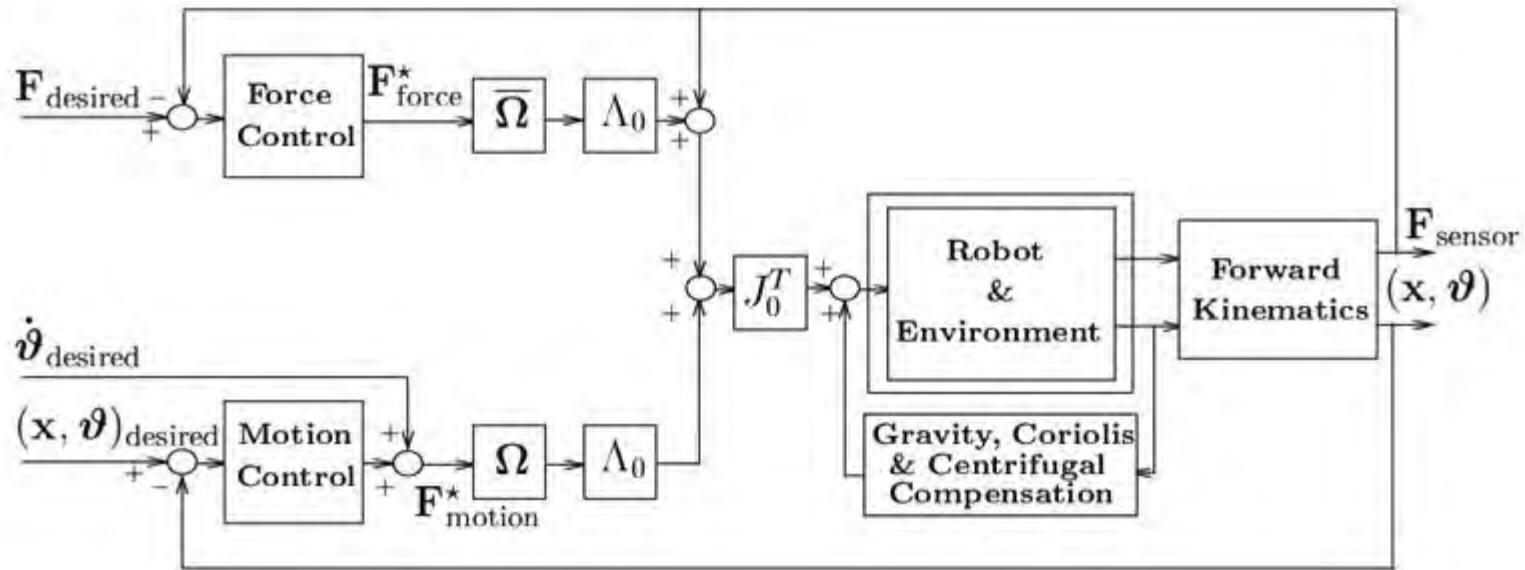
Two decoupled Subsystems
