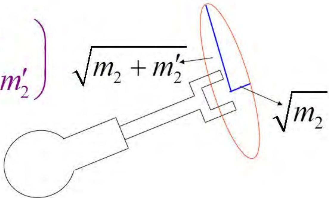
$${}^0 \Lambda = \begin{pmatrix} m_2 + m'_2 s l^2 & -m'_2 s c l \\ -m'_2 s c l & m_2 + m'_2 c l^2 \end{pmatrix}$$
