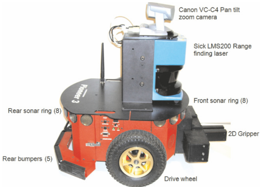
Fig. 1.3 Pioneer P3-DX sensors and actuators
