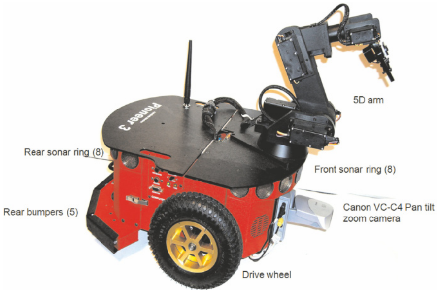
Fig. 1.4 Pioneer P3-DX sensors and actuators, alternative configuration
