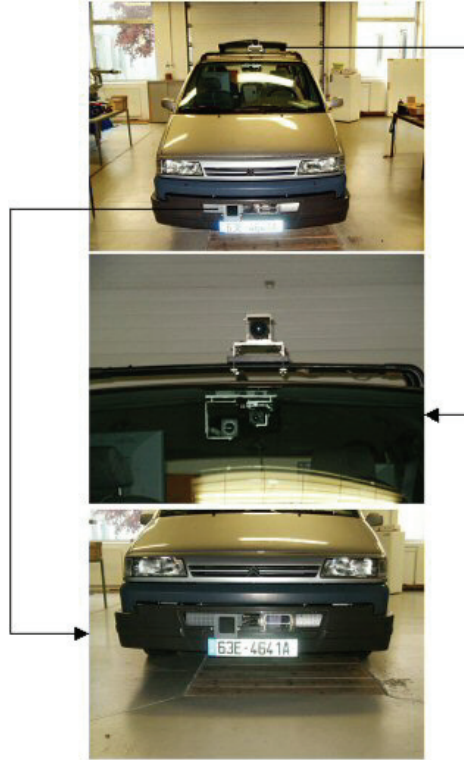
Fig. 1. LASMEA's experimental vehicle exteroceptive sensors.
