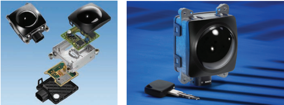
Fig. 6. Bosch 2 nd Generation Long Range Radar Sensor Unit
