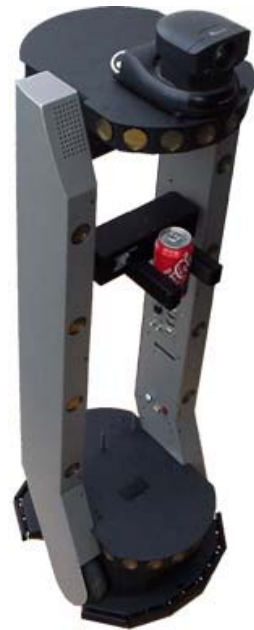
Figure 6. The Performance PeopleBot sports an attractive body design and bundled systems, including voice synthesis and recognition for human-interaction research and applications.
