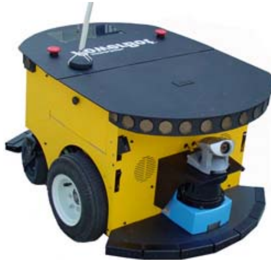
Figure 7. PowerBot™ carries over 100 kg of payload.
