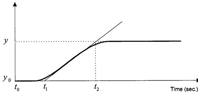
**Figure 3.3: Plant step response in Z-N method**
