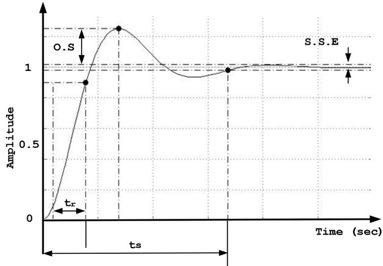
**Figure 3.5: Unit step response curve showing  $t_r$ ,  $t_s$ ,  $O.S$  and  $SSE$**
