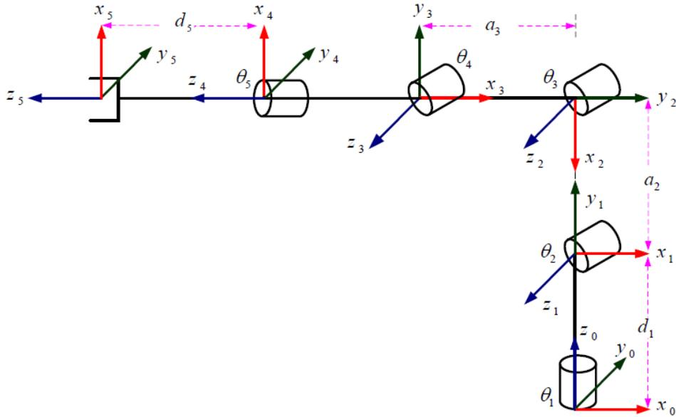
**Figure 6.2: Frame assignment for the Lynx 6 robot arm.**
