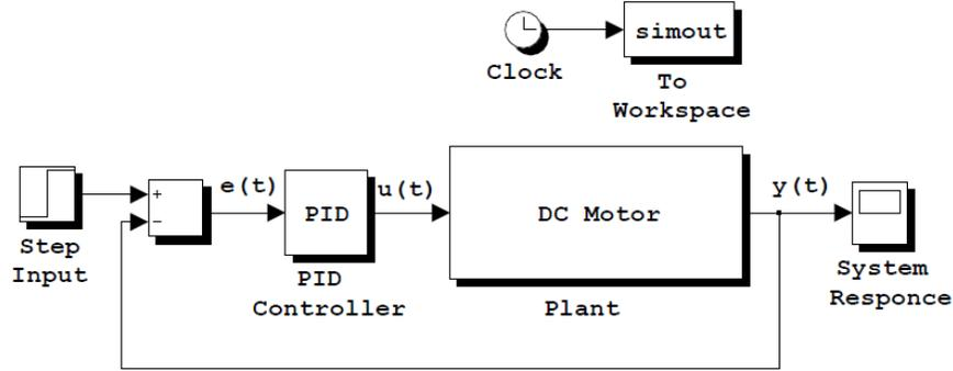
**Figure 3.4: SIMULINK model of PID controller**
