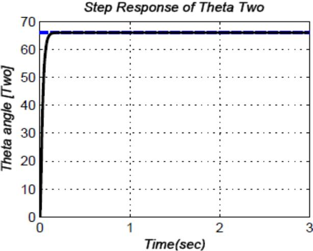
Figure 6.5: PID control step response for  $\theta_1, \theta_2$
