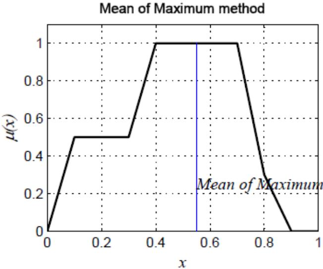
**Figure C.3: Mean of Max defuzzification method**
