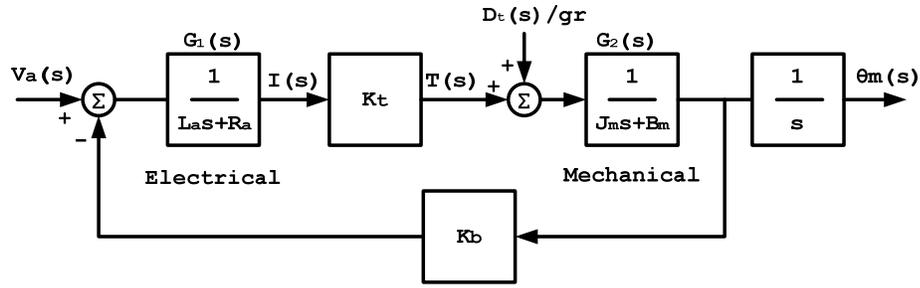
**Figure 2.3: Block diagram for DC motor system**
