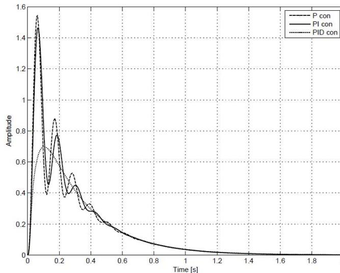
**Figure 3.7: Transient response to step disturbance input**
