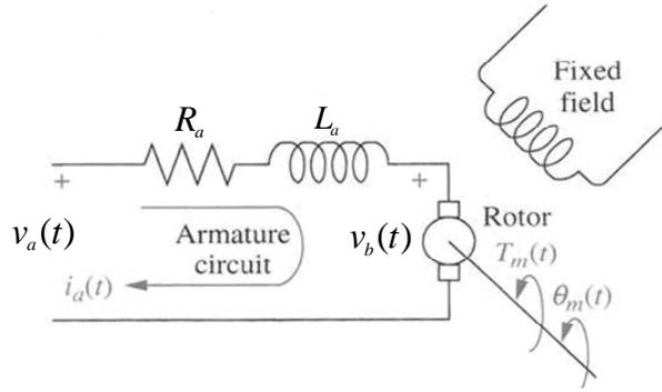
**Figure 2.2: Schematic of DC motor system**
