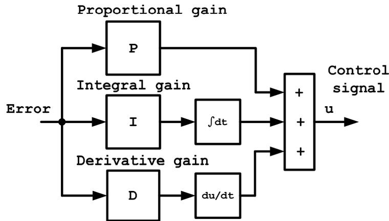
**Figure 3.1: PID controller structure**
