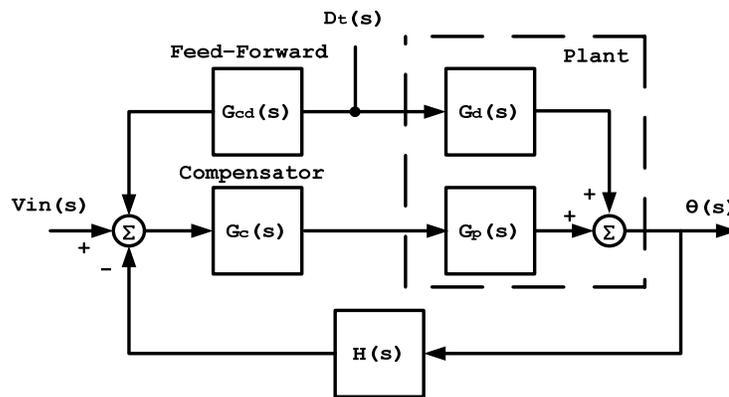
**Figure 3.10: Feedforward compensation**
