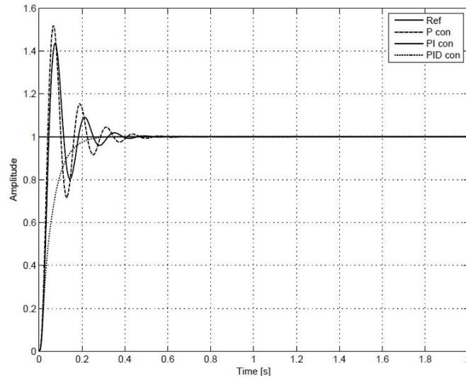
**Figure 3.6: Transient response to step reference input**
