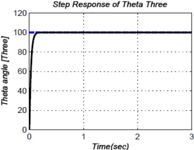
Figure 6.6: PID control step response for  $\theta_3$
