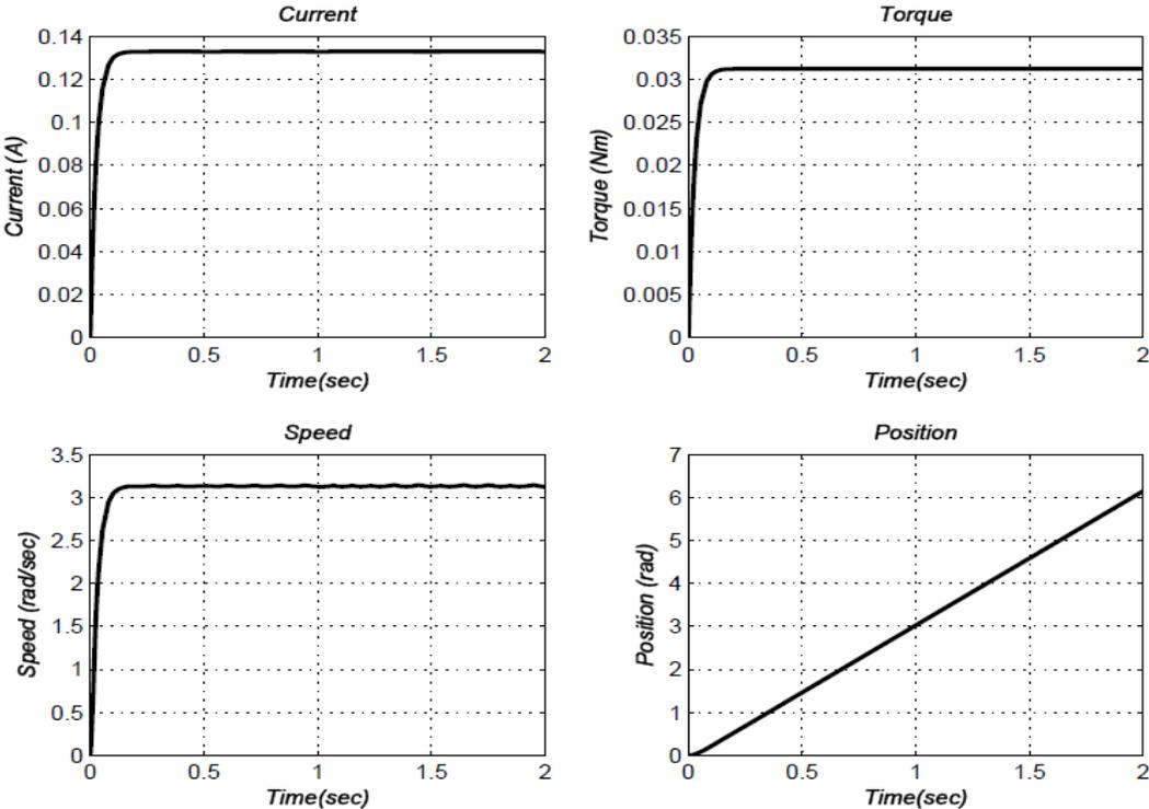
Figure 2.5: DC motor open loop step response without load
