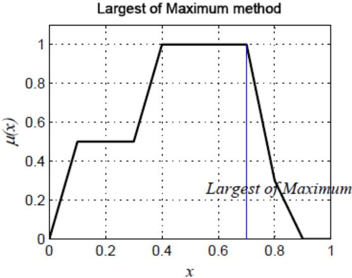
**Figure C.4: Largest of Maximum defuzzification method**
