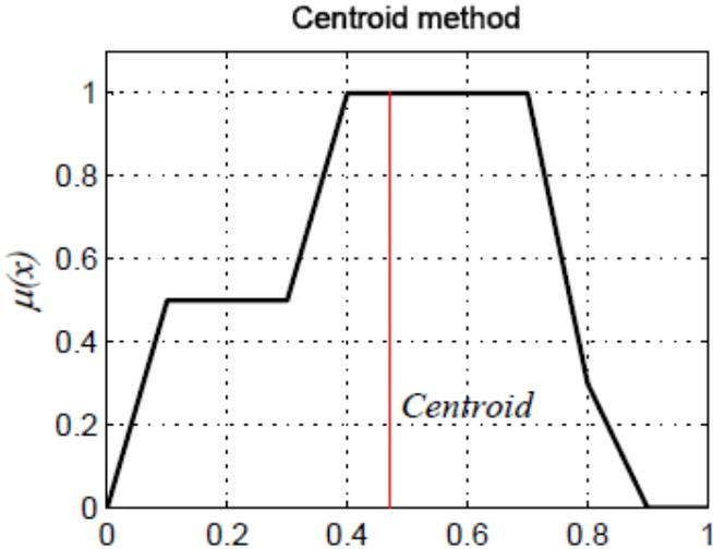
Figure C.1: Centroid defuzzification method
