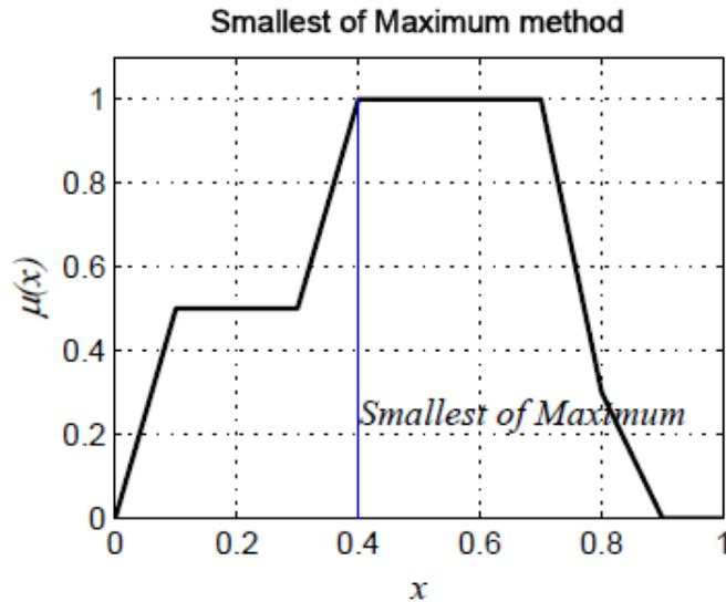
Figure C.5: Smallest of Maximum defuzzification method
