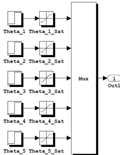
**Figure 3.13: Input angles with saturation boundaries**
