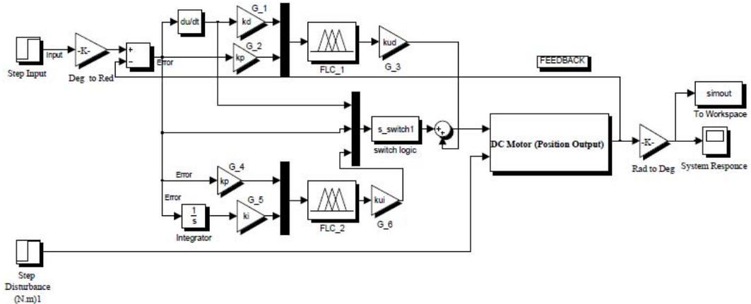
**Figure D.2: Fuzzy PID controller**
