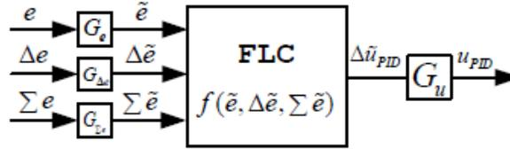
**Figure 4.12: Three input fuzzy PID (Type I)**
