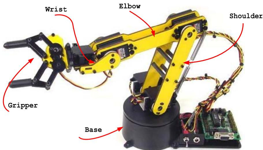
**Figure 6.1: Lynx6 robot arm**
