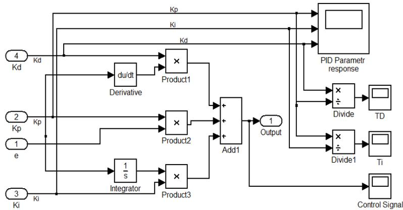
**Figure D.4: PID controller**
