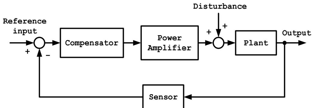
**Figure 1.3: The basic structure of (SISO) system**
