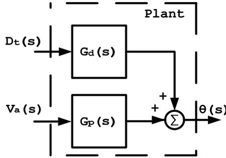
**Figure 3.8: Servomotor model**
