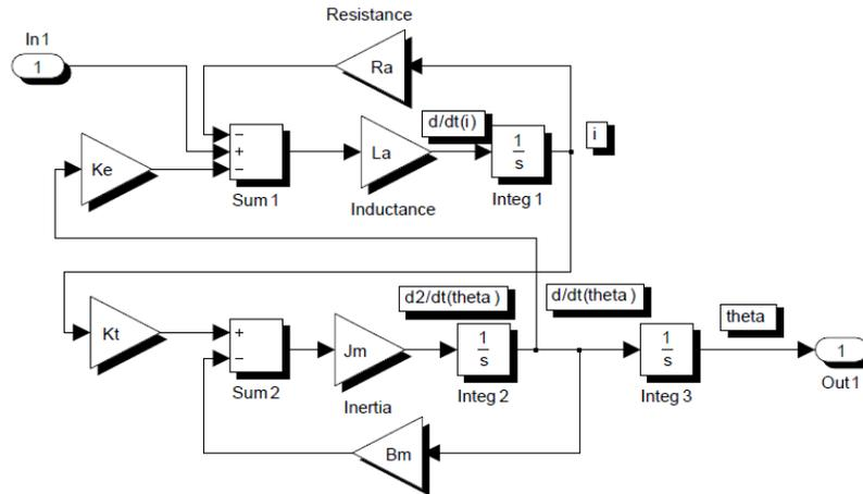
**Figure 2.4: DC motor subsystem using SIMULINK**
