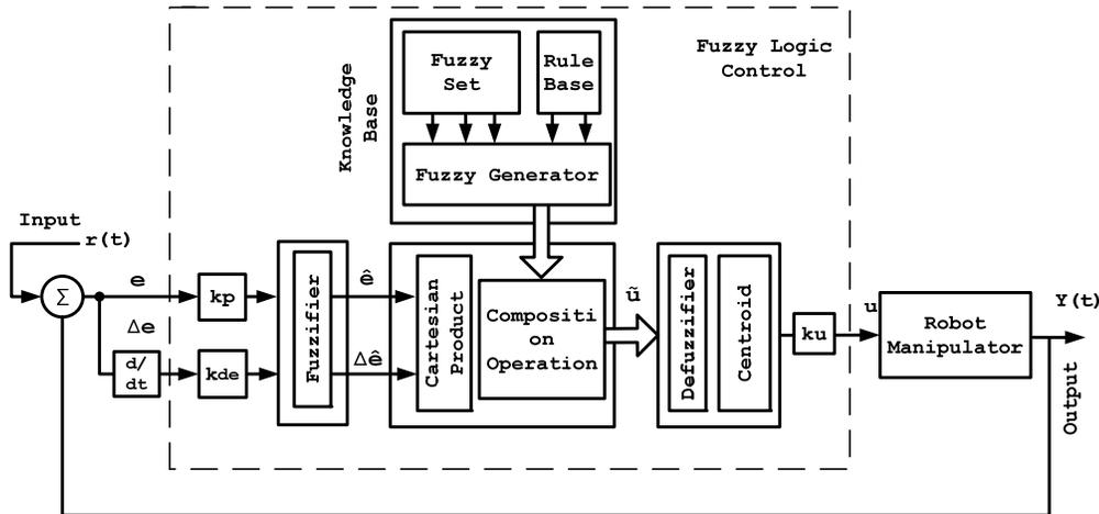
**Figure 4.6: Fuzzy control system structure**
