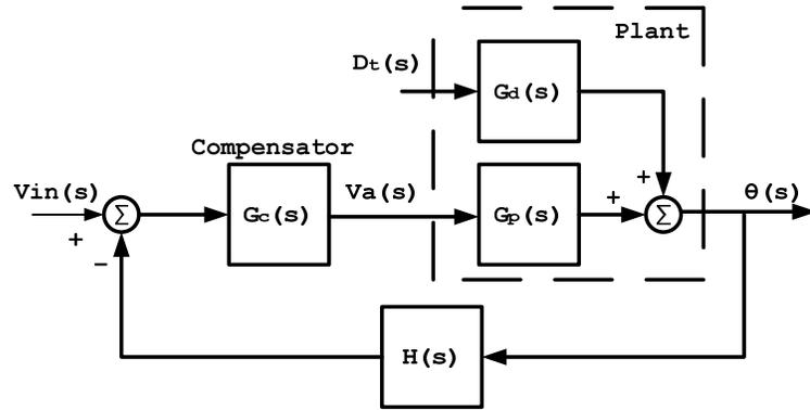
**Figure 3.9: Closed loop system with disturbance input**
