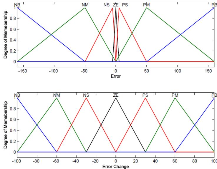
**Figure 4.8: Membership function for inputs  $e$  and  $\Delta e$**
