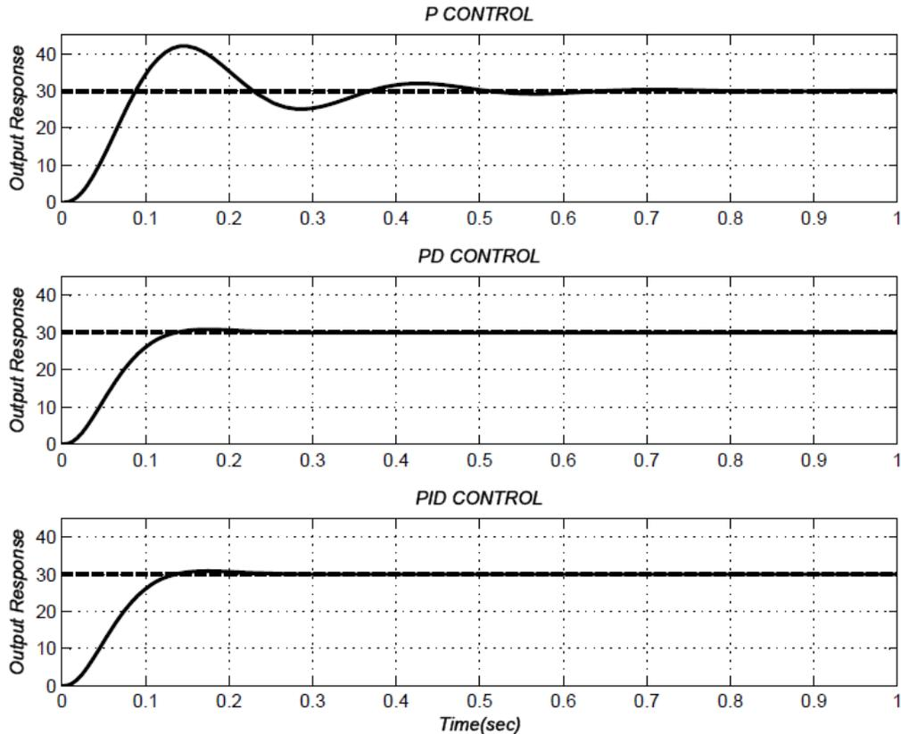
Figure 3.2: Step response of P, PD, and PID controllers
