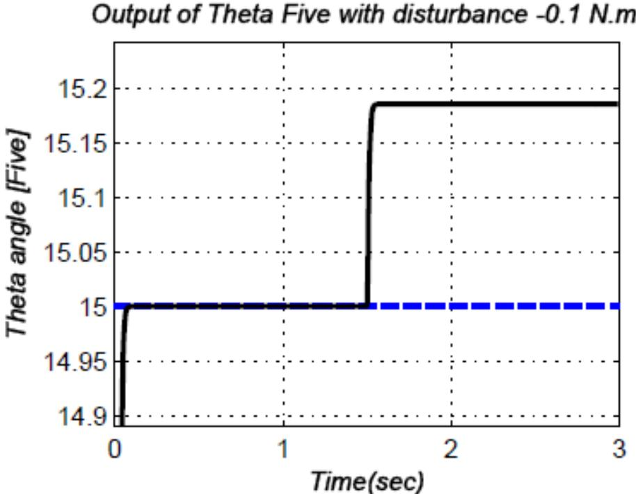
Figure 6.9: Output with disturbance for  $\theta_5$
