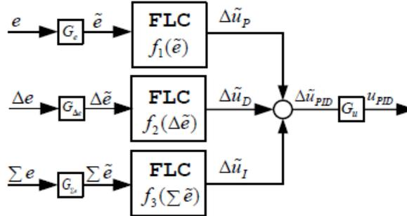
**Figure 4.13: Three input fuzzy PID (Type II)**
