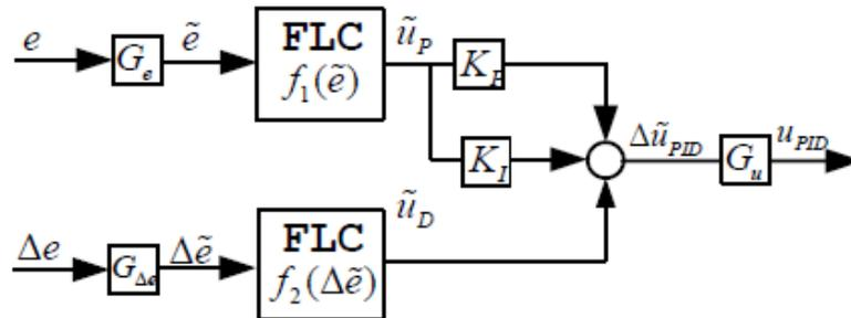
**Figure 4.15: Two input fuzzy PID (Type II)**
