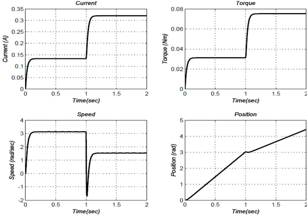
Figure 2.6: DC motor model simulation with load disturbance
