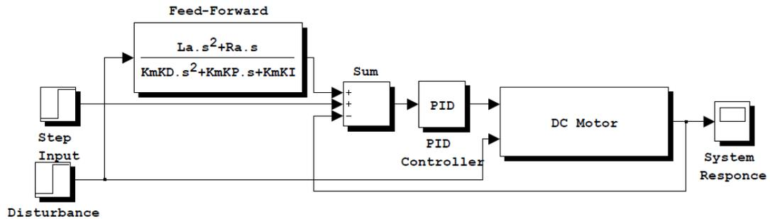
**Figure 3.11: PID controller with feedforward compensator**
