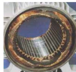
Figure 1. Electric motor winding shorted. Source: [4].
