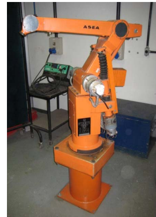
Figure 3. ASEA ROBOT IRB6, year of manufacture 1977. Source: [7].
