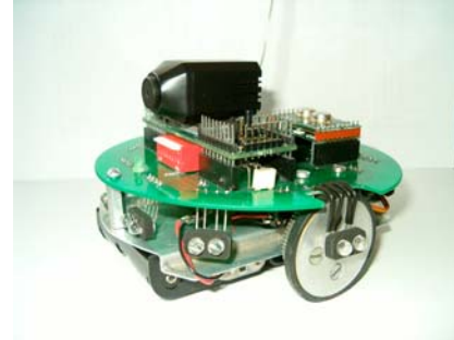
Our proto board and Turtle robot equipped in wireless color camera
