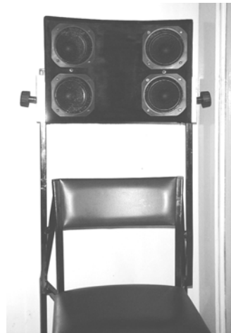
Fig. II.8. The active headrest system.
