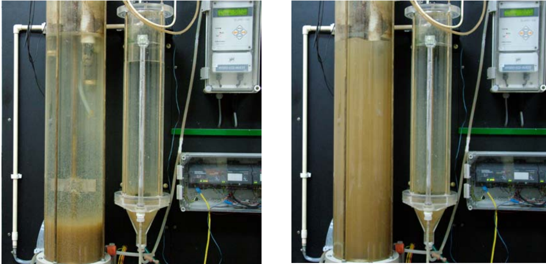
Fig.6. Presentation of the biomass manipulations. After the thickened sludge is pumped from the settler into the reactor, which results in a drop of level in the settler (right image) and a corresponding rise of level in the reactor, a new set point level is determined and reached by the controller. Mixing in the reactor starts (left image) and the system restarts its normal continuous operation with a changed biomass concentration.
