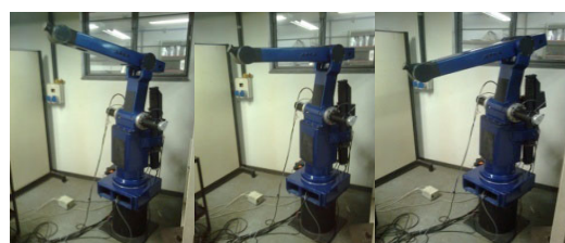
Fig.10. G-Code generated in MATLAB® controlling joint movements through Mach 3®.
