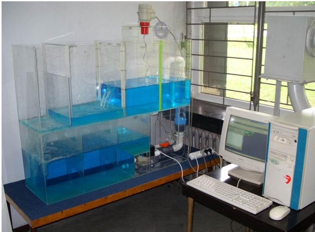
Fig. 71. Installation for the flow-rate measurement in the open channel.
