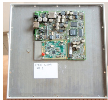
Fig. 2. Casing for CPE with PCB
