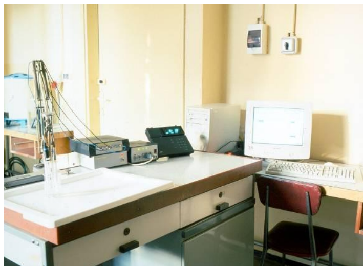
Fig. 51. The measuring set-up for multi-component ion-selective measurements.
