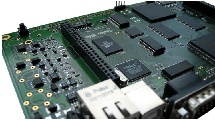
Fig. 6. One of the DSP platforms designed and realised in the Measurements and Control Systems Division in the Institute of Automatic Control.
