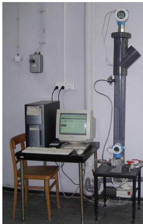
Fig. 72. Laboratory stand for investigation of properties of level transducers.
