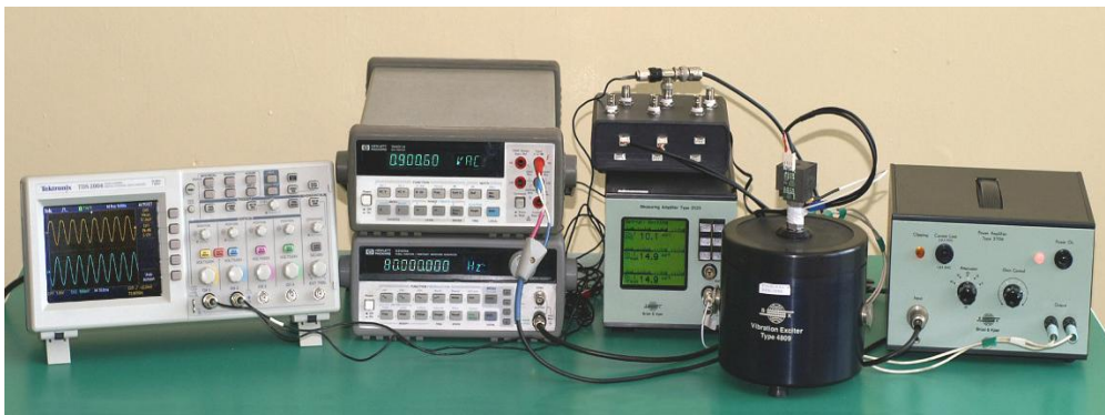
Fig. 45. View of the calibration set-up for frequency range 20Hz – 20kHz.
