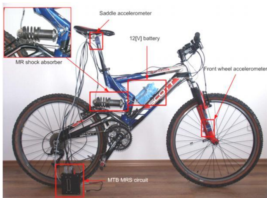
Fig. 32. Semi-active vibration damping system.
