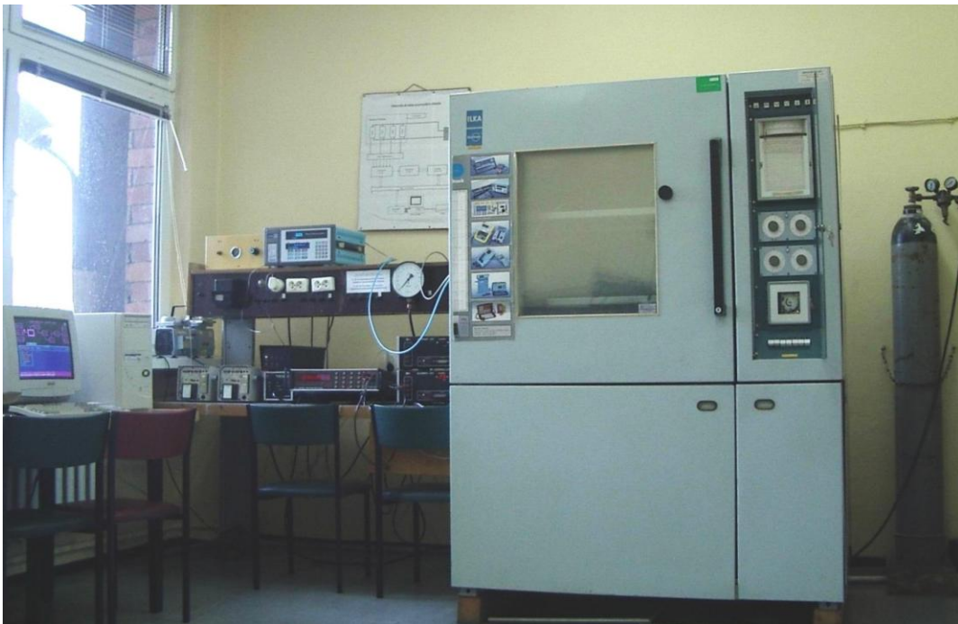
Fig. 48. Calibration system for pressure sensors and transmitters.
