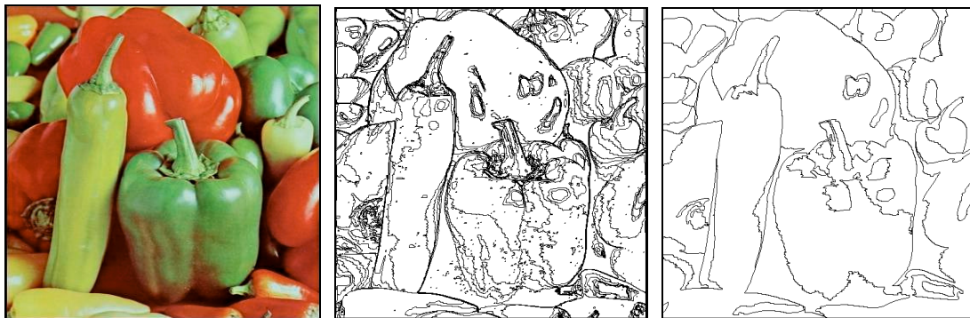
Fig. 2. Example of segmentation results in RGB colour space for image Peppers: original image (left), parameter value: d=30 (middle), parameter values: d=60 , A=500 (right).
