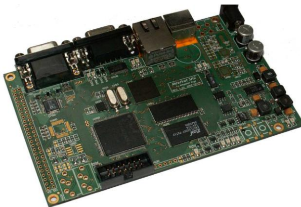
Fig. 5. Evaluation board of educational starter kit for Renesas SH7619 microcontroller.
