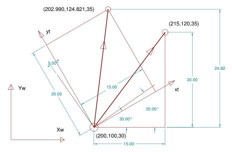
Figure 9: World and tool coordinate move in the X-Y plane
