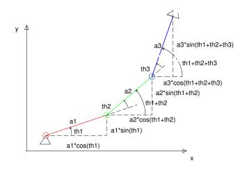
Figure 3: x- and y-components of links
