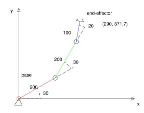
Figure 5: Example 2: Planer 3-dof serial arm
