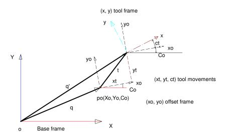
Figure 8: Tool coordinate move in the X-Y plane
