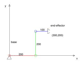
Figure 4: Example 1: Planer 3-dof serial arm
