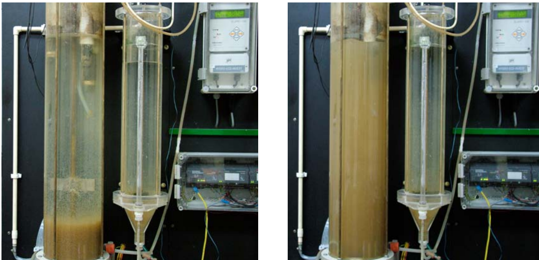
Fig.6. Presentation of the biomass manipulations. After the thickened sludge is pumped from the settler into the reactor, which results in a drop of level in the settler (right image) and a corresponding rise of level in the reactor, a new set point level is determined and reached by the controller. Mixing in the reactor starts (left image) and the system restarts it's normal continuous operation with a changed biomass concentration.
