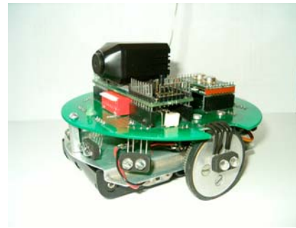
Our proto board and Turtle robot equipped in wireless color camera
