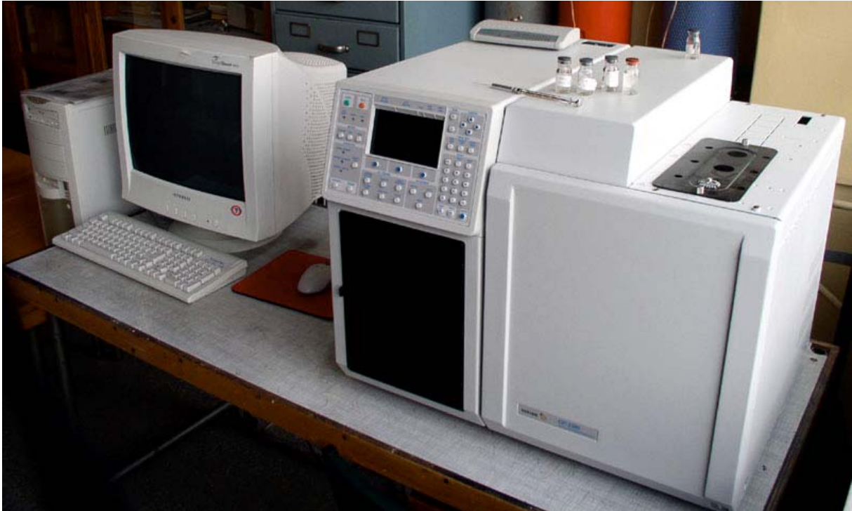
Fig. 1. Chromatographic stand with Varian 3800 Gas Chromatograph
