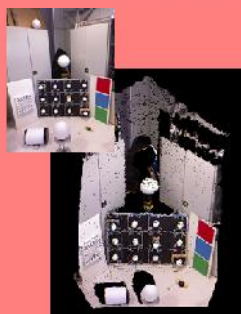
Scene volume 2m x 2m x 3m Theoretical precisions variable in the range [7,35] mm
