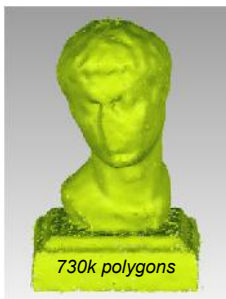
KINECT at 50cm (theoretical \sigma_z \approx 0.7 mm)
