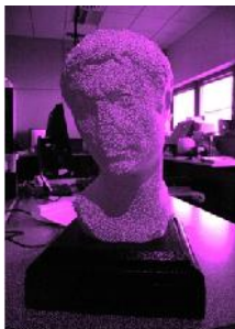
KINECT at 50cm (theoretical \sigma_z \approx 0.7 mm)
