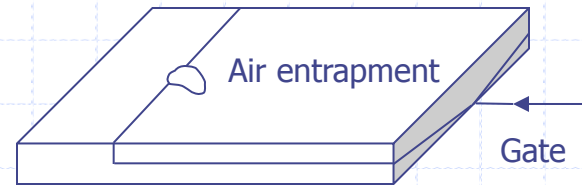
Edge gate: warp free, air entrapment
