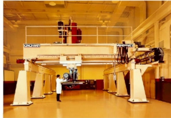
Fig 1.0 Tape Layer Configuration and Axis of Movement
