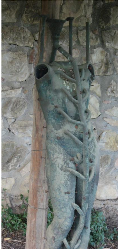
Etruscan casting with runners circa 500 BCE
